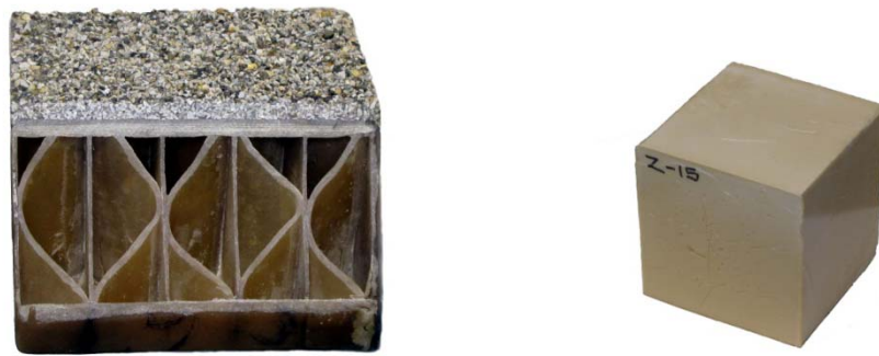
(a) Current Honeycomb Structure (b) Polyurethane Foam Core Alternative
