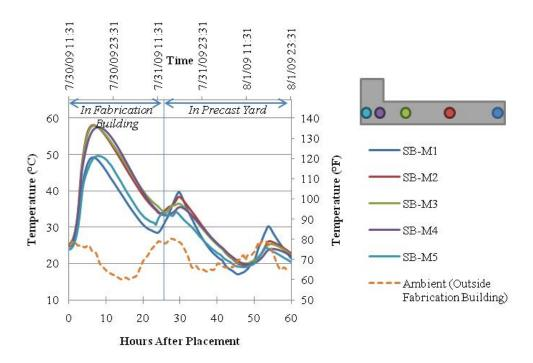
Figure 8.4. Hydration Temperature of HS-SCC Spandrel Beam at Mid-Span.
