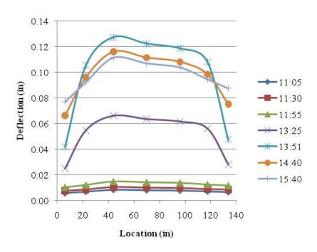
Figure F.4. Adjustments to HSC Deck Panel with GFRP for Thermal Effects.
