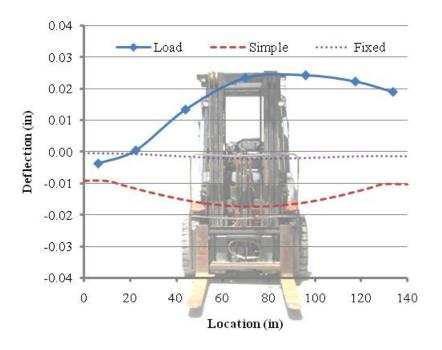
Figure H.10. HSC GFRP Reinforced Deck Panel Deflection – Load Case E.
