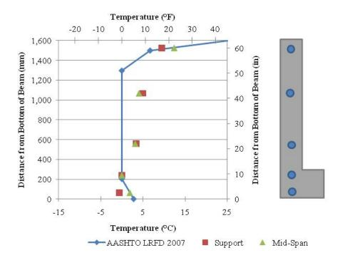
Figure 8.29. Design Positive Gradients vs. HS-SCC Maximum Positive Gradients.
