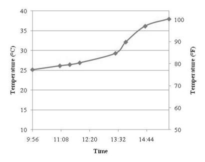
Figure 11.8. HSC Beam Temperature during Load Testing.
