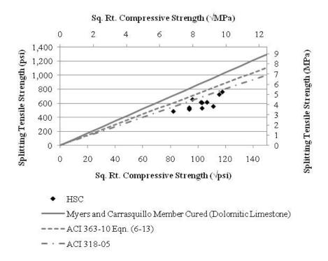
Figure 7.10. Splitting Tensile Strength vs. Compressive Strength of HSC.
