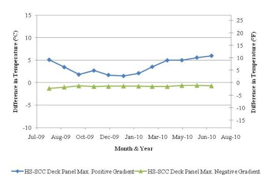
b.) HS-SCC Deck PanelsFigure 8.23. Average Maximum Monthly Gradients of Bridge Deck Panels.
