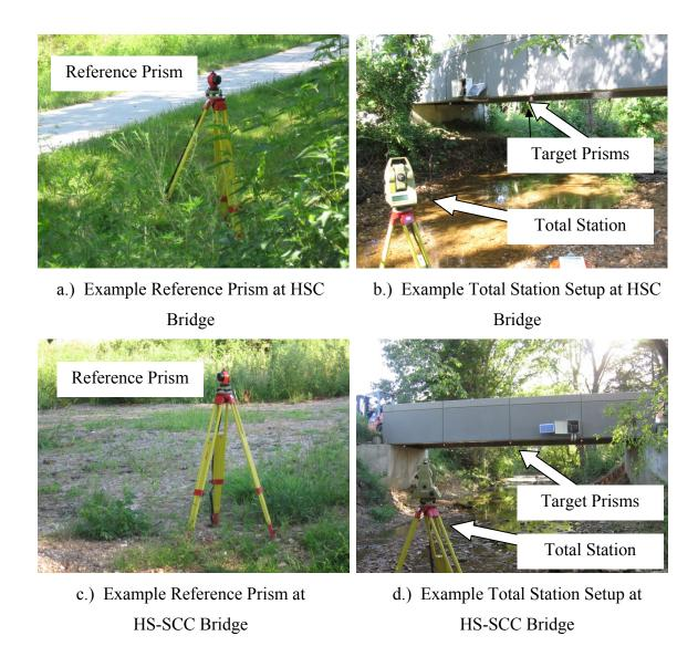
Figure 11.4. Total Station Test Setup.
