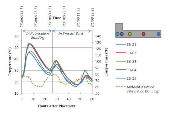
Figure 8.3. Hydration Temperature of HS-SCC Spandrel Beam at Support.
