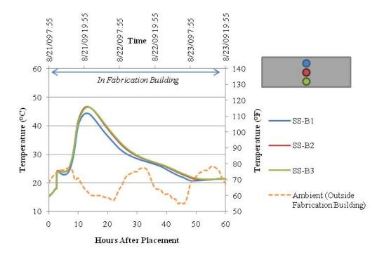
Figure 8.8. Hydration Temperature of HS-SCC Deck Panel Reinforced with GFRP.
