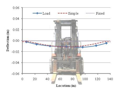
Figure 11.17. HS-SCC GFRP Reinforced Deck Panel Deflection – Load Case F.
