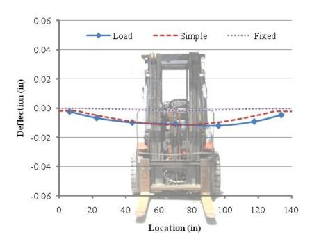
Figure I.11. HS-SCC GFRP Reinforced Deck Panel Deflection – Load Case F.
