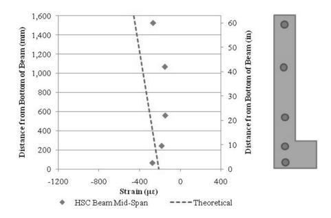
Figure 9.23. Strain Profile after Deck Placement for HSC Beam.
