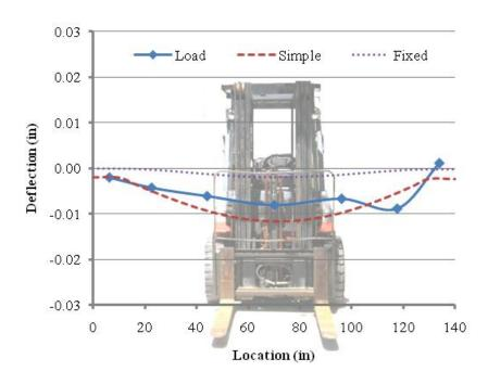
Figure 11.15. HS-SCC Mild Steel Reinforced Deck Panel Deflection – Load Case D.
