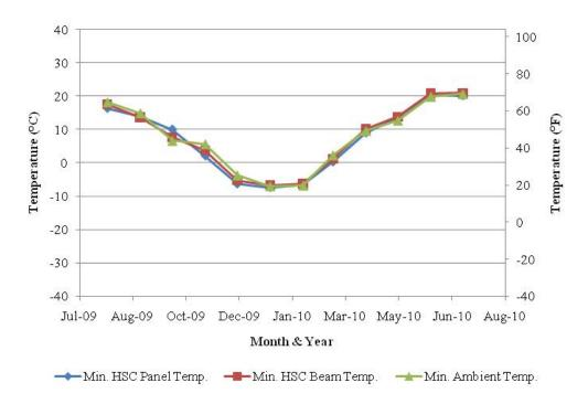
Figure 8.16. Average Minimum Monthly Temperature of HSC Bridge.
