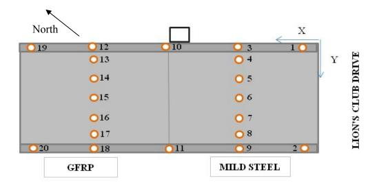
Figure 11.5. Target Prisms on HSC Bridge.
