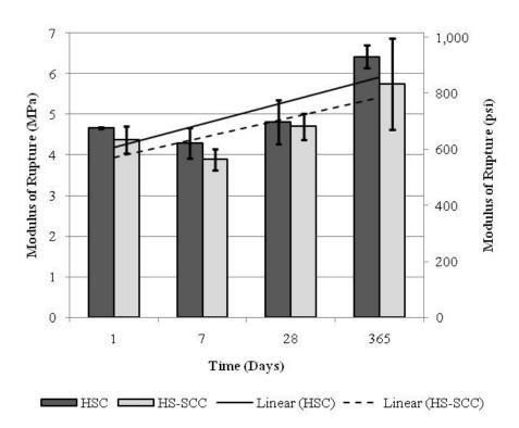
Figure 7.6. Average Modulus of Rupture for HSC & HS-SCC.
