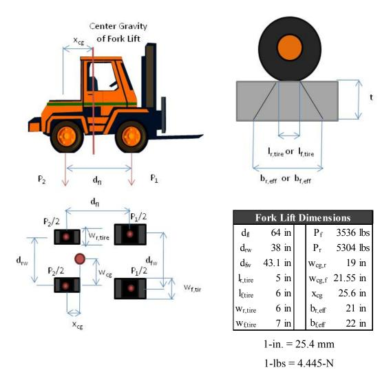
Figure 11.1. Fork Lift Dimensions for Live Load Test.
