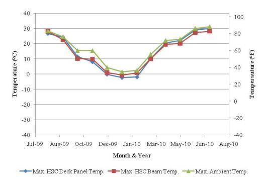
Figure 8.14. Average Maximum Monthly Temperature of HSC Bridge.
