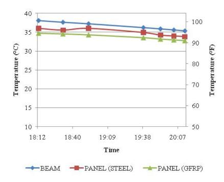
Figure F.5. Internal Temperature vs. Time for HS-SCC Bridge during Load Testing.
