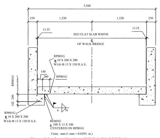
Figure 3.2. Cross Section of HSC & HS-SCC Bridges.
