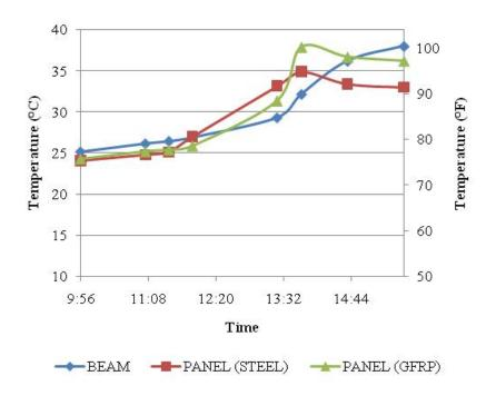
Figure F.1. Internal Temperature vs. Time for HSC Bridge during Load Testing.
