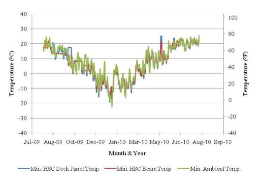
Figure 8.12. Minimum Daily Temperature of HSC Bridge.
