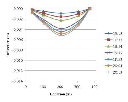
Figure 11.11. HS-SCC Beam Adjustments due to Temperature to Baseline Reading.
