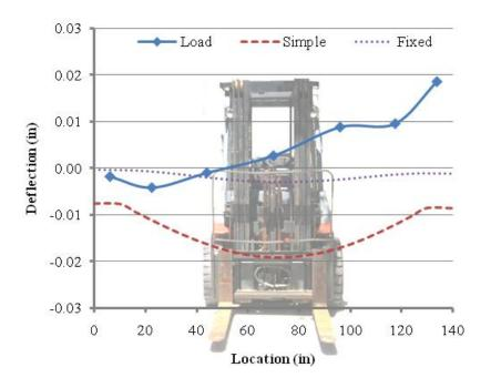
Figure H.8. HSC Mild Steel Reinforced Deck Panel Deflection – Load Case D.
