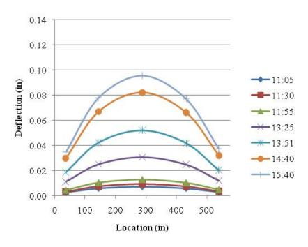
Figure F.2. Adjustments to HSC Beam for Thermal Effects.
