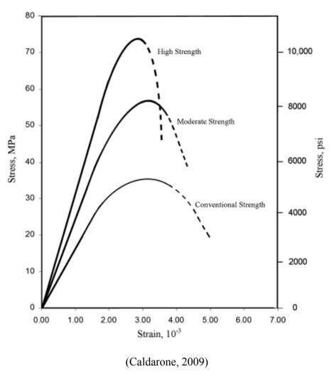
Figure 2.1. Stress Strain Relationships for Varying Concrete Strengths.
