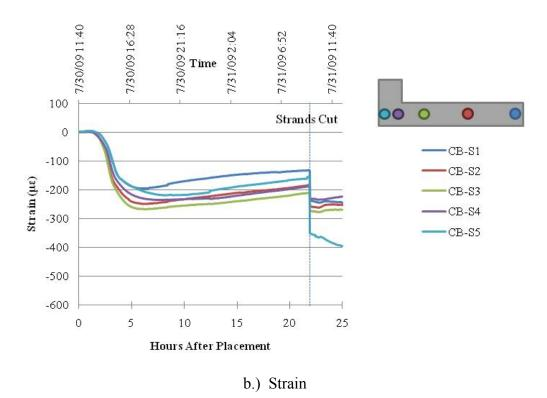
Figure 9.1. Strains & Temperatures at Support of HSC Beam during Fabrication.
