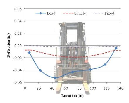
Figure H.11. HSC GFRP Reinforced Deck Panel Deflection – Load Case F.
