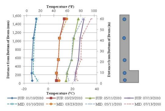
Figure 8.25. Thermal Gradients in HS-SCC Spandrel Beams.
