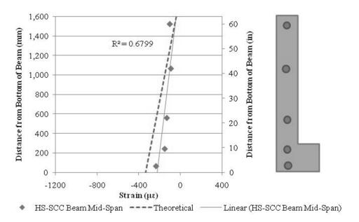
Figure 9.11. Strain of HS-SCC Spandrel Beam at 7 Days.
