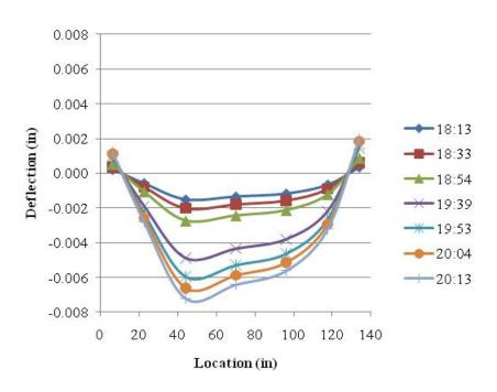
Figure F.8. Adjustments to HS-SCC Deck Panel with GFRP for Thermal Effects.
