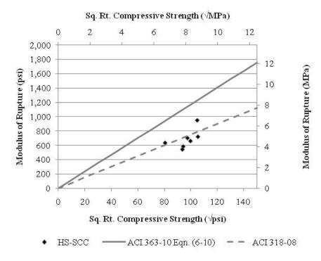
Figure 7.8. Modulus of Rupture vs. Compressive Strength for HS-SCC.
