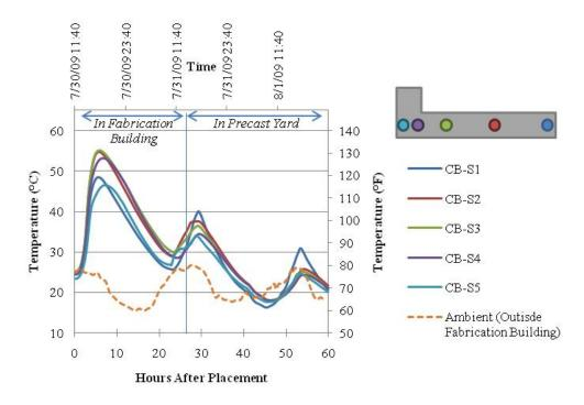
Figure 8.1. Hydration Temperature of HSC Spandrel Beam at Support.
