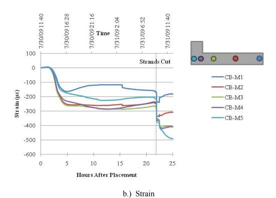
Figure 9.2. Strains & Temperatures at Mid-Span of HSC Beam during Fabrication.
