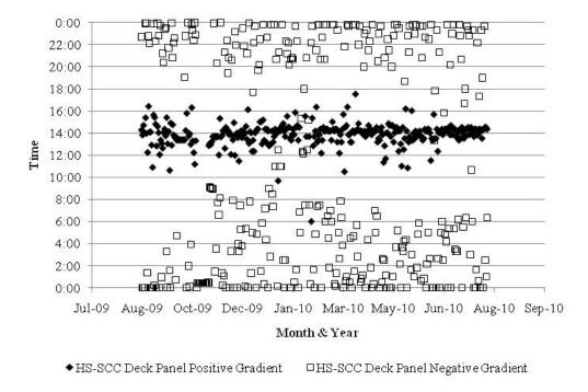
Figure 8.21. Time of Maximum Positive & Negative Gradients for HS-SCC Panels.
