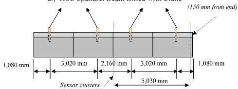
e.) HS-SCC Spandrel Beam Lifted with Crane
