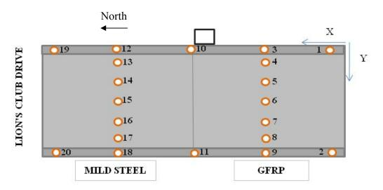
Figure 11.6. Target Prisms on HS-SCC Bridge.
