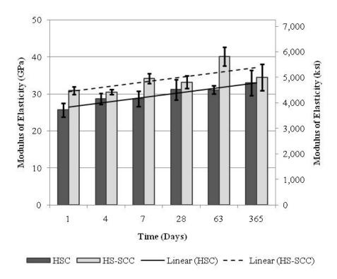
Figure 7.3. Average Modulus of Elasticity for HSC & HS-SCC.
