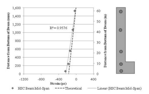
Figure 9.5. Strain Comparison at Mid-Span of HSC Spandrel Beam at Release.
