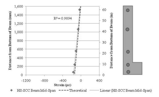
Figure 9.6. Strain Comparison at Mid-Span of HS-SCC Spandrel Beam at Release.
