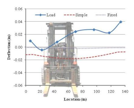
Figure H.5. HSC GFRP Reinforced Deck Panel Deflection – Load Case B.
