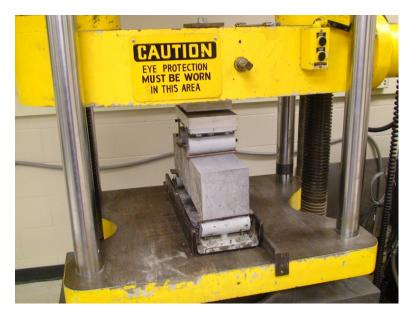
Figure 5.5. Modulus of Rupture.
