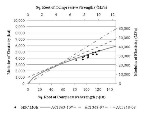
Figure 7.4. Modulus of Elasticity vs. Compressive Strength for HSC.
