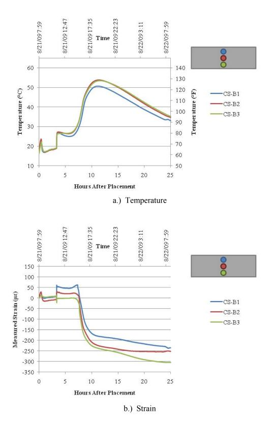
Figure 9.14. Strain in HSC Deck Panel Reinforced with GFRP.
