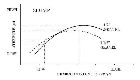
Figure 2.2. Concrete Strength to Cement Content to Aggregate Size (Myers, 1998).
