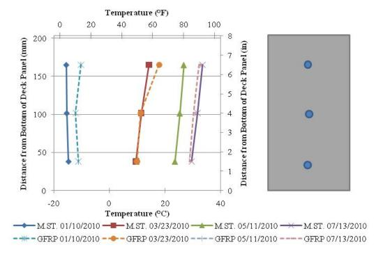
Figure 8.27. Thermal Gradients in HS-SCC Precast Deck Panels.
