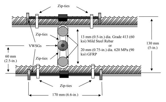
Figure 6.16. Schematic of VWSGs Attached to Deck Panel Reinforcement.
