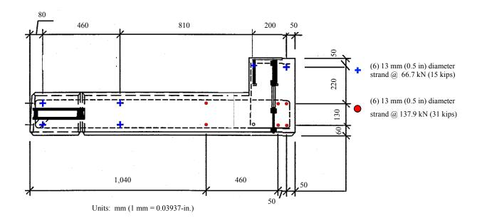
Figure 3.3. Cross Section of HSC & HS-SCC Bridge Spandrel Beam.
