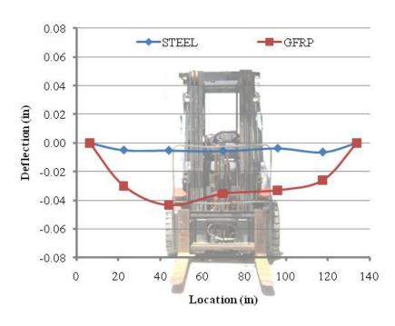
Figure 11.20. HSC Deck Panel with Steel vs. GFRP Deflection – Load Case D & F.
