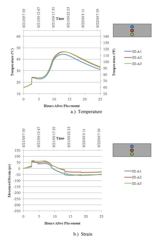
Figure 9.15. Strain in HS-SCC Deck Panel Reinforced with Mild Steel.
