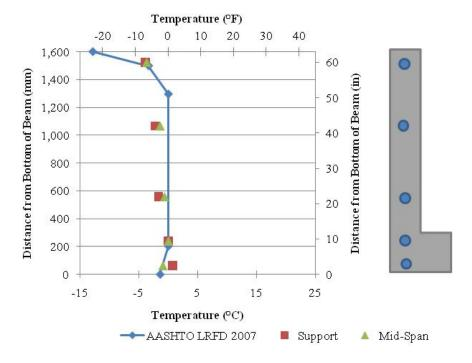
Figure 8.31. Design Negative Gradients vs. HS-SCC Maximum Negative Gradients.
