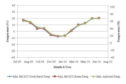
Figure 8.17. Average Minimum Monthly Temperature of HS-SCC Bridge.
