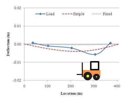
Figure I.1. HS-SCC Instrumented Beam Deflection – Load Case A.
