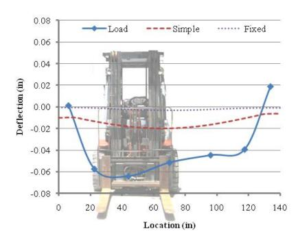
Figure H.7. HSC GFRP Reinforced Deck Panel Deflection – Load Case C.
