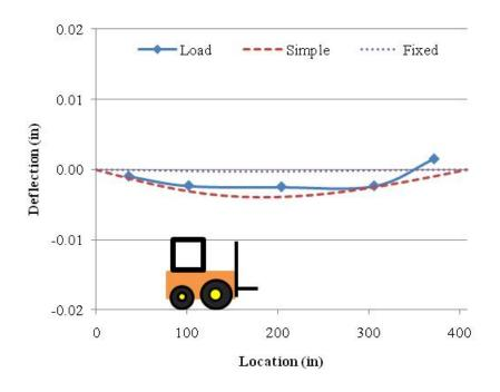
Figure I.6. HS-SCC Instrumented Beam Deflection – Load Case C.
