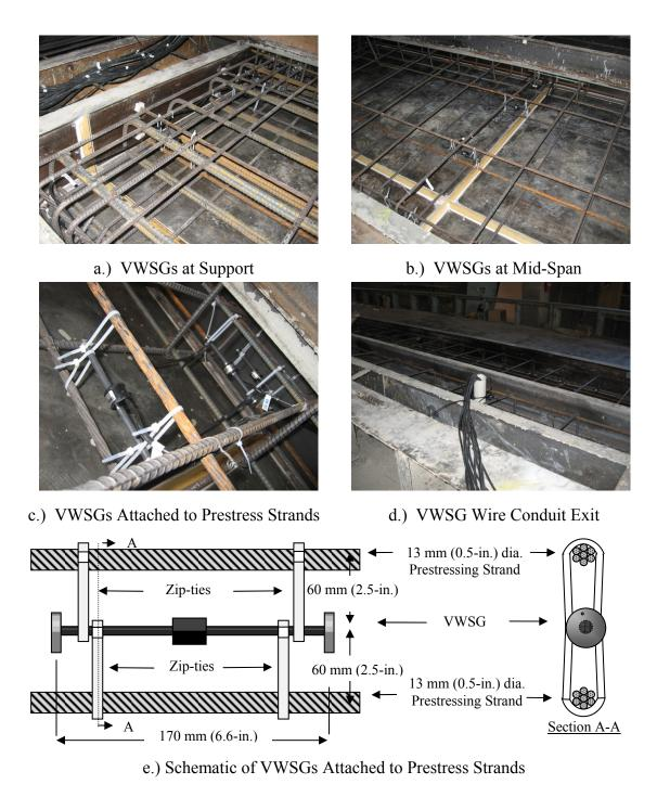
Figure 6.13. VWSGs in Beams at Fabrication in Marshall, MO.
