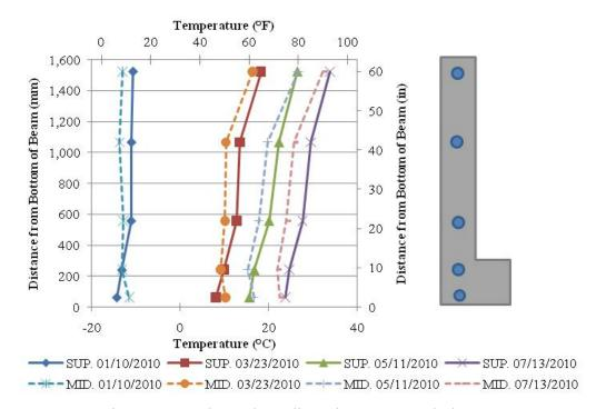
Figure 8.24. Thermal Gradients in HSC Spandrel Beams.
