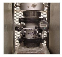
Figure 5.4. Modulus of Elasticity Test.
