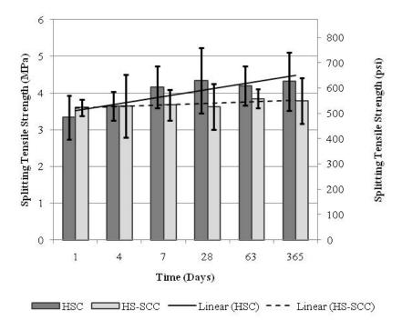
Figure 7.9. Average Splitting Tensile Strength of HSC & HS-SCC.
