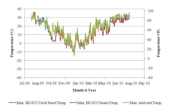
Figure 8.11. Maximum Daily Temperature of HS-SCC Bridge.
