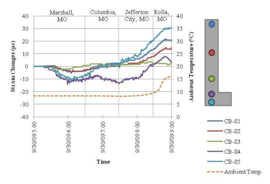
Figure 9.19. Support Strain Changes during Transportation of HSC Spandrel Beam.
