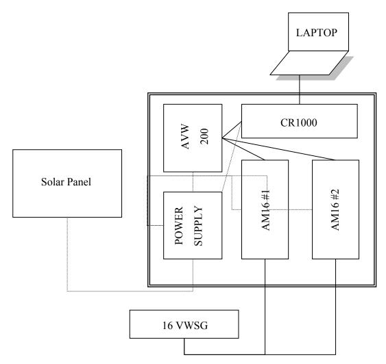
Figure 6.6. DAS Components & Gauges for Each Bridge.
