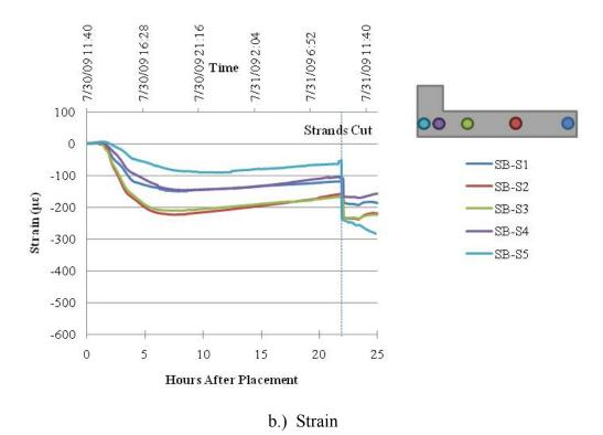
Figure 9.3. Strains & Temperatures at Support of HS-SCC Beam during Fabrication.
