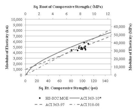
Figure 7.5. Modulus of Elasticity vs. Compressive Strength for HS-SCC.
