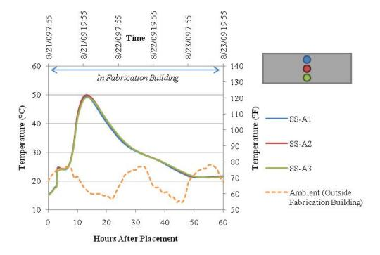
Figure 8.7. Hydration Temperature of HS-SCC Deck Panel Reinforced with Mild Steel.
