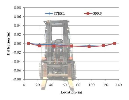
Figure 11.21. HS-SCC Deck Panel with Steel vs. GFRP Deflection – Load Case A & C.
