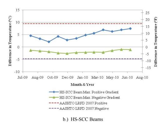
Figure 8.22. Average Maximum Monthly Gradients of Bridge Beam.
