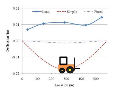
Figure H.3. HSC Instrumented Beam Deflection – Load Case B.
