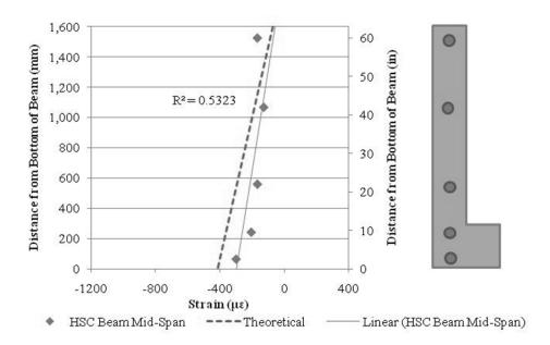
Figure 9.10. Strain at Mid-Span of HSC Spandrel Beam at 14 Days.
