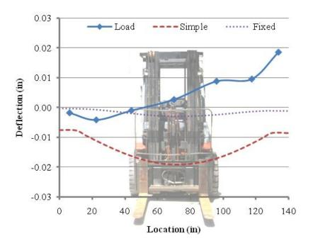
Figure 11.14. HSC Mild Steel Reinforced Deck Panel Deflection – Load Case D.
