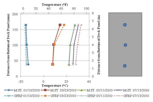
Figure 8.26. Thermal Gradients in HSC Precast Deck Panels.
