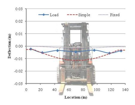
Figure I. 9. HS-SCC Mild Steel Reinforced Deck Panel Deflection – Load Case E.
