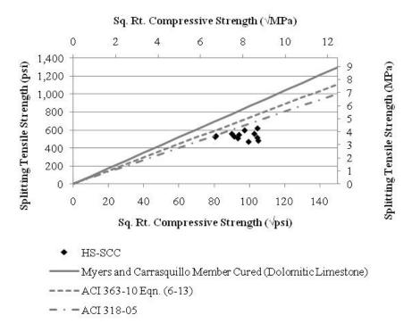
Figure 7.11. Splitting Tensile Strength vs. Compressive Strength of HS-SCC.
