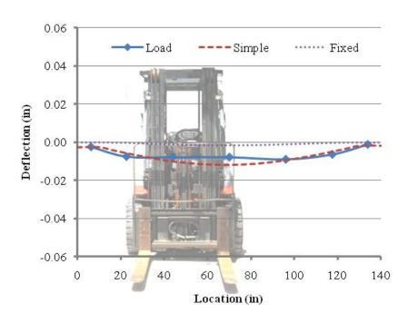
Figure I.7. HS-SCC GFRP Reinforced Deck Panel Deflection – Load Case C.
