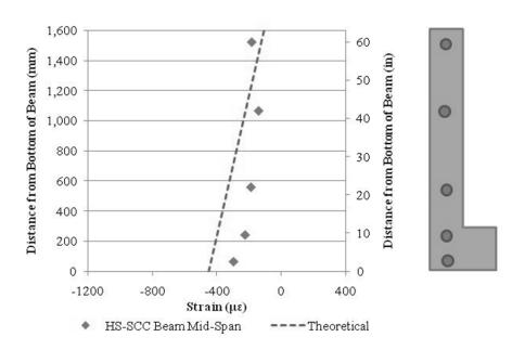
Figure 9.24. Strain Profile after Deck Placement of HS-SCC Beam.
