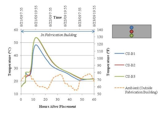
Figure 8.6. Hydration Temperature of HSC Deck Panel Reinforced with GFRP.
