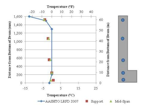
Figure 8.30. Design Negative Gradients vs. HSC Maximum Negative Gradients.
