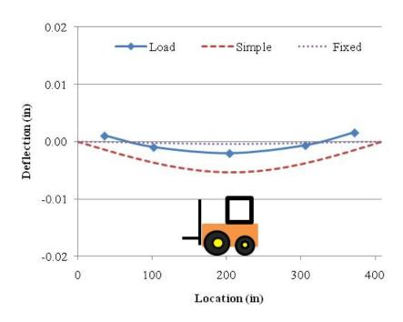
Figure I.3. HS-SCC Instrumented Beam Deflection – Load Case B.
