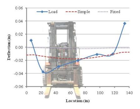
Figure H.4. HSC Mild Steel Reinforced Deck Panel Deflection – Load Case B.
