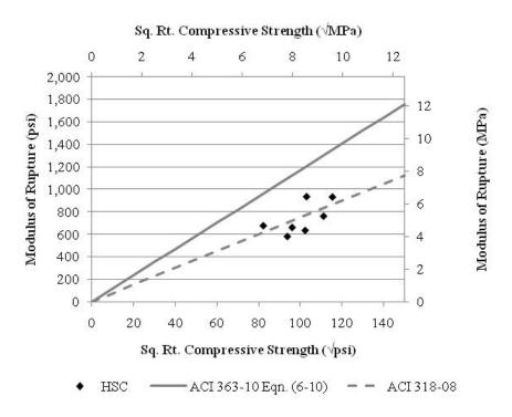
Figure 7.7. Modulus of Rupture vs. Compressive Strength for HSC.
