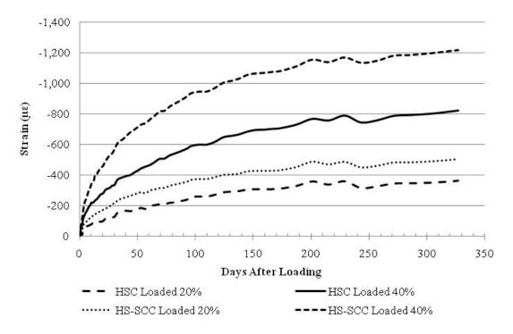
Figure 7.12. Creep Results for HSC & HS-SCC.
