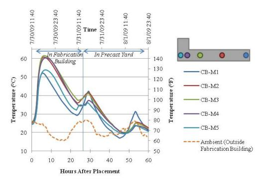
Figure 8.2. Hydration Temperature of HSC Spandrel Beam at Mid-Span.
