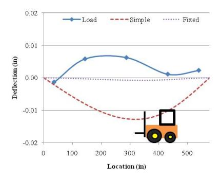
Figure H.6. HSC Instrumented Beam Deflection – Load Case C.
