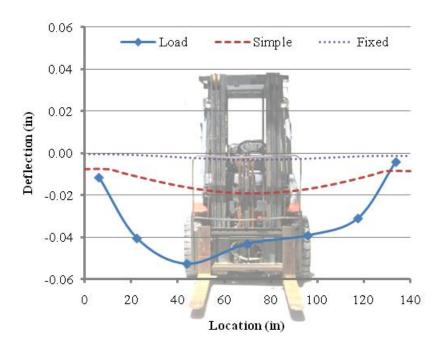
Figure 11.16. HSC GFRP Reinforced Deck Panel Deflection – Load Case F.
