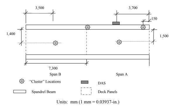
Figure 6.8. Plan Illustrating HSC Instrumentation "Cluster" Locations (Plan View).
