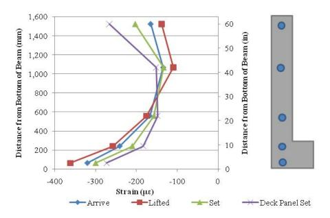
Figure 9.21. HSC Mid-Span Spandrel Beam Strain Profile during Erection.
