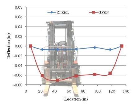
Figure 11.19. HSC Deck Panel with Steel vs. GFRP Deflection – Load Case A & C.
