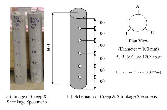
Figure 5.7. Creep & Shrinkage Specimens & DEMEC Point Arrangements.
