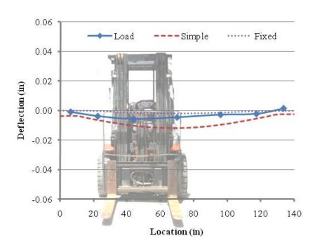
Figure I.5. HS-SCC GFRP Reinforced Deck Panel Deflection – Load Case B.
