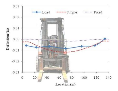
Figure I.2. HS-SCC Mild Steel Reinforced Deck Panel Deflection – Load Case A.
