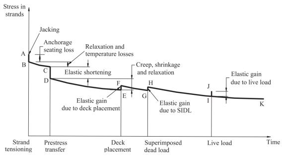
Figure 2.4. Stress vs. Time for Bridge Girder (Tadros et. al., 2003).
