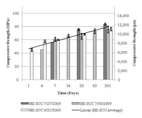
Figure 7.2. HS-SCC Average Compressive Strength.
