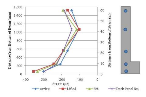
Figure 9.22. HS-SCC Mid-Span Spandrel Beam Strain Profile during Erection.
