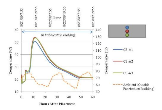
Figure 8.5. Hydration Temperature of HSC Deck Panel Reinforced with Mild Steel.
