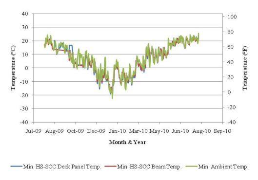
Figure 8.13. Minimum Daily Temperature of HS-SCC Bridge.
