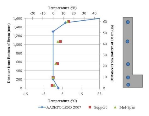
Figure 8.28. Design Positive Gradients vs. HSC Maximum Positive Gradients.
