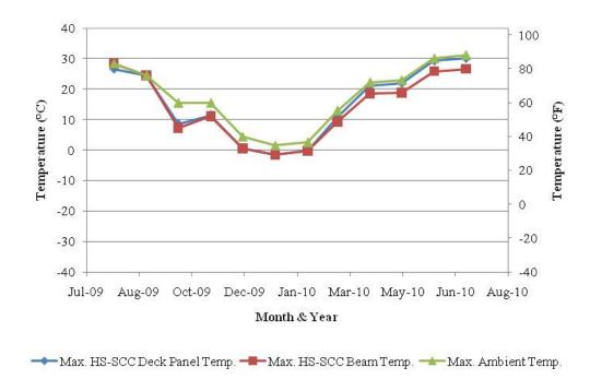
Figure 8.15. Average Maximum Monthly Temperature of HS-SCC Bridge.
