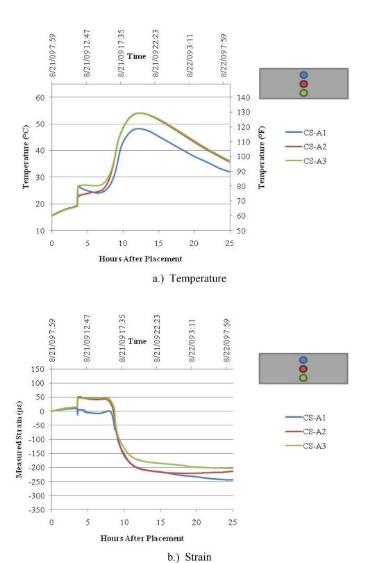
Figure 9.13. Strain in HSC Deck Panel Reinforced with Mild Steel.
