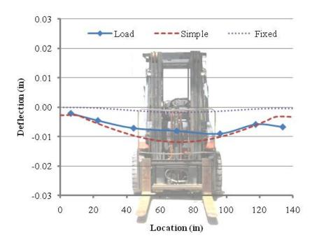
Figure I.10. HS-SCC GFRP Reinforced Deck Panel Deflection – Load Case E.
