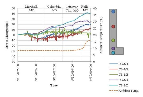
Figure 9.20. Mid-Span Strain Changes during Transportation of HSC Spandrel Beam.
