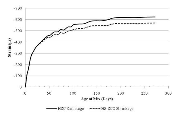
Figure 7.13. Shrinkage Results for HSC & HS-SCC Precast Deck Panels.
