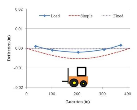
Figure 11.13. HS-SCC Spandrel Beam Deflection – Load Case B.
