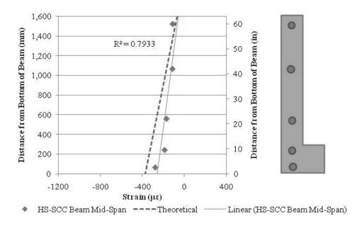
Figure 9.12. Strain of HS-SCC Spandrel Beam at 14 Days.
