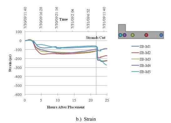
Figure 9.4. Strains & Temperatures at Mid-Span of HS-SCC Beam during Fabrication.
