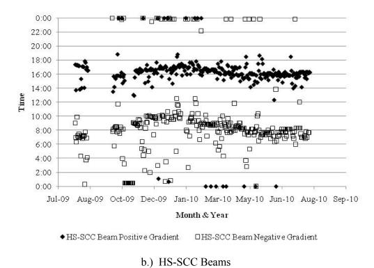
Figure 8.20. Time of Maximum Positive & Negative Gradients for Beams.
