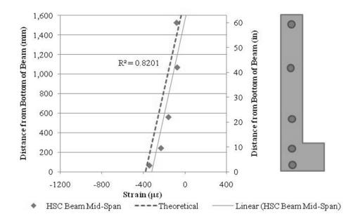
Figure 9.9. Strain at Mid-Span of HSC Spandrel Beam at 7 Days.
