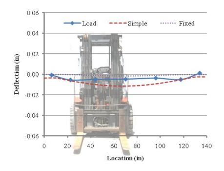
Figure I.4. HS-SCC Mild Steel Reinforced Deck Panel Deflection – Load Case B.
