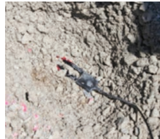
Strain gage anchored to rebar and moisture gage embedded in subgrade soil
