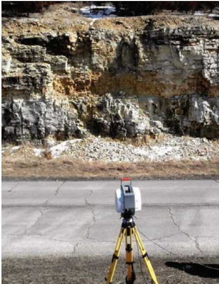
Figure 1: LIDAR scanner measuring rock cut
