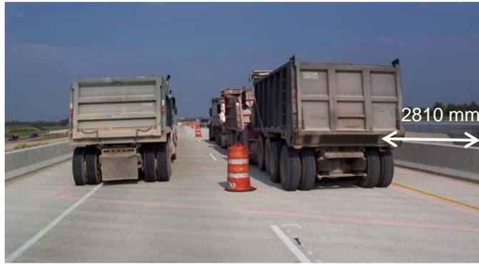
Figure 20 Trucks Aligned on Test 1
