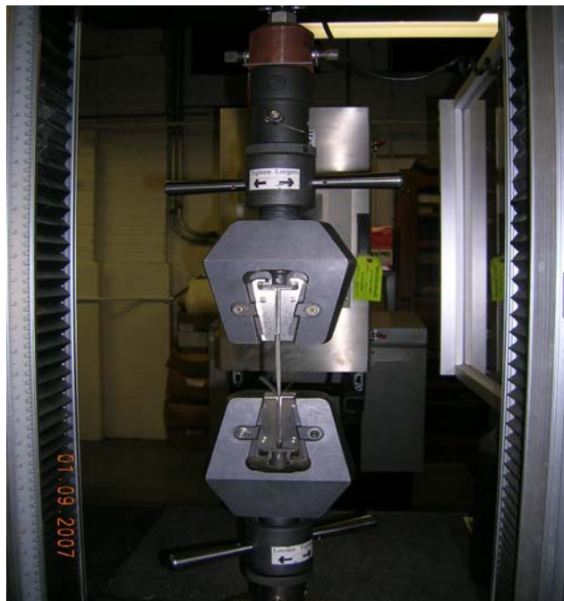
Figure 3.29. The Tensile Test Setup for the Latex Membranes
