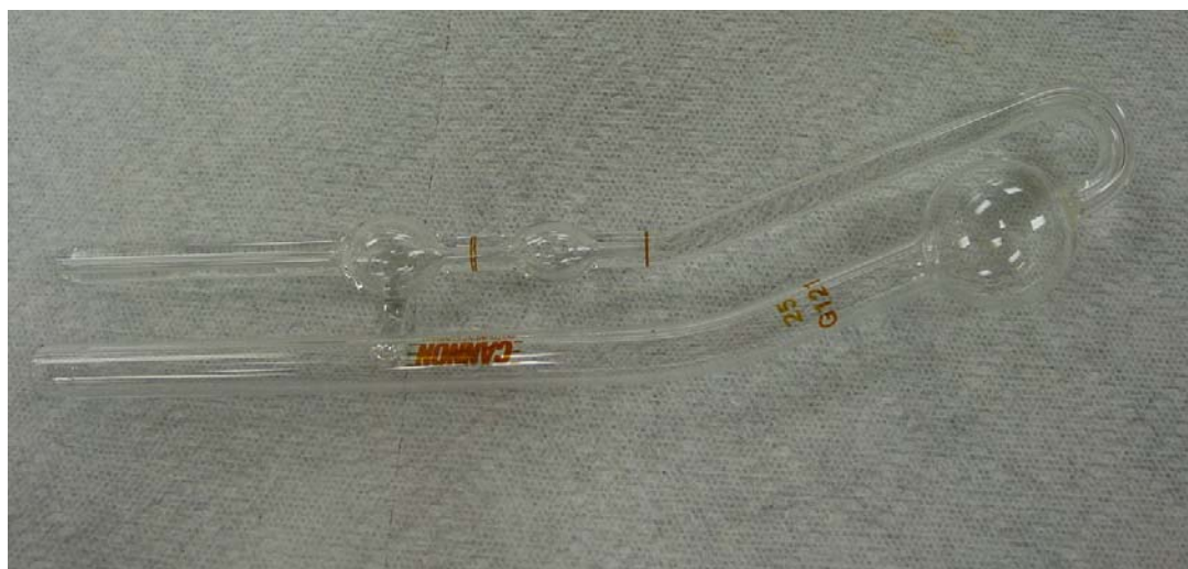
Figure 3.14. The Cannon-Fenske Viscometer Tube, No. 25
