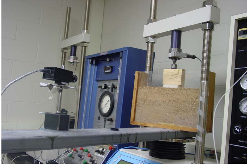
Figure 5.10. Experiment Setup for the Rectangular Footing
