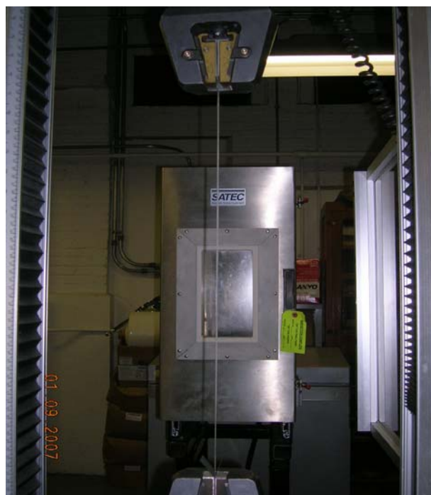
Figure 3.30. The Typical Testing Results for the Membrane of Low Degradation (The specimen can be stretched to six times its original length)
