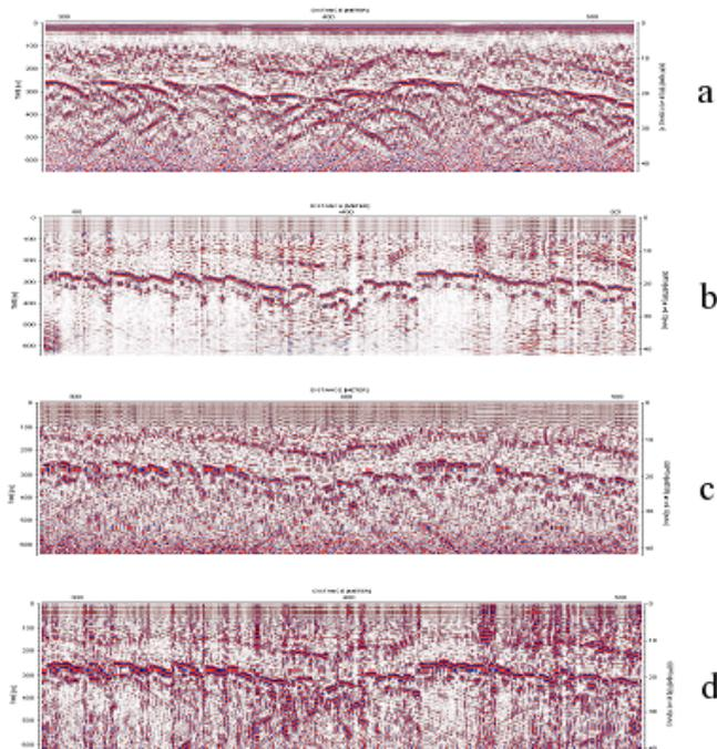
Fig.16. Comparison of quality of different migration algorithms: a – row data; b – diffraction stack; c – Kirchhoff migration; d – Stolt fk migration. It can be seen that the clearest image is produced with a simple diffraction stack, but Kirchhoff algorithm provides with more details. Stolt migration effectively restores the geometry of main boundaries but generates more artifacts at the noisy data.
