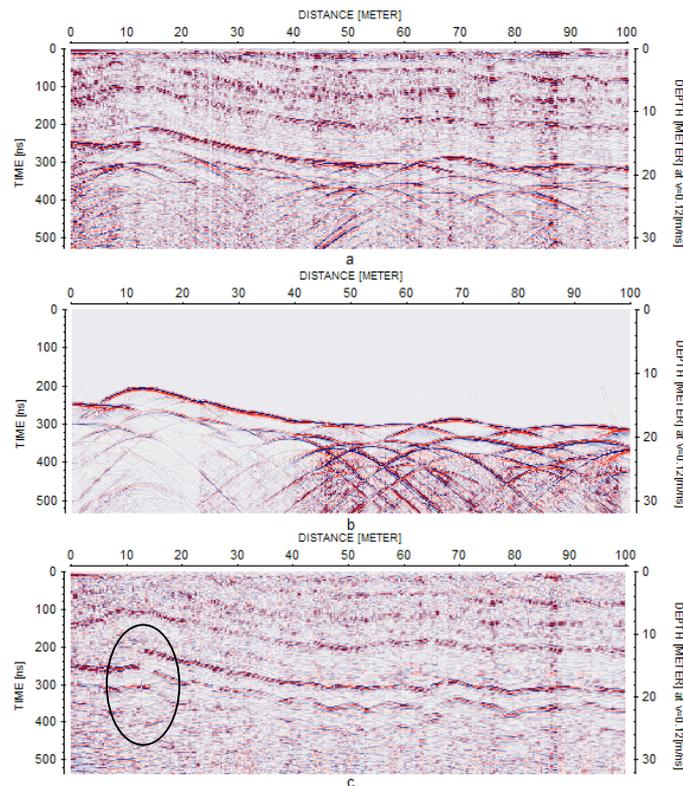
Fig. 12. GPR data inversion comprised the picking the desired horizon at the migrated section (c) to construct the initial model, iterative modeling (b) to fit the successive model to unmigrated data (a). In this case the resulting model of the marker clay layer complicated with a fault( identified by circle) clearly coincides with a raw record.
