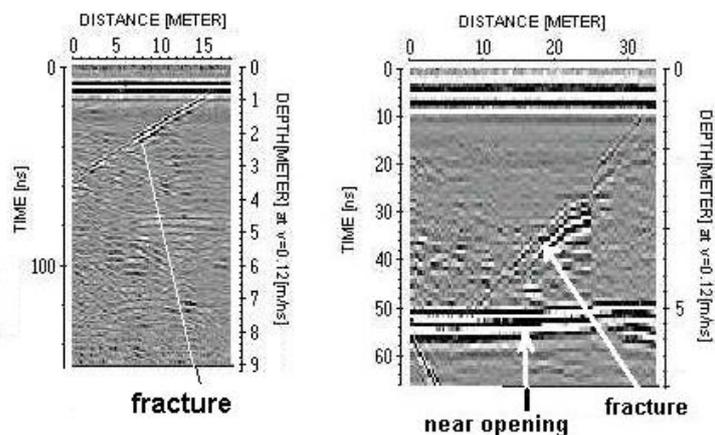
Fig. 17. Images of the open fractures into the pillars of room 166.
