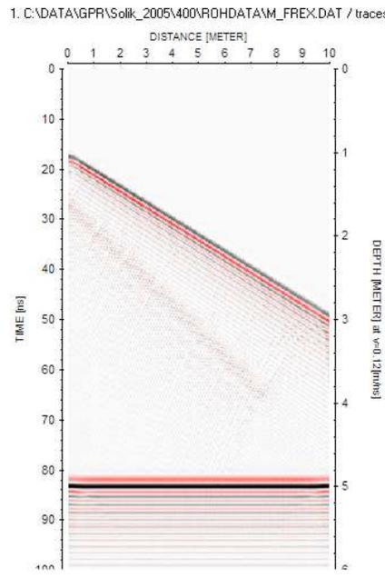
*Fig. 13. Model of sounding of the mine pillar with millimetric scale fracture of dip angle of 25 degree.*
