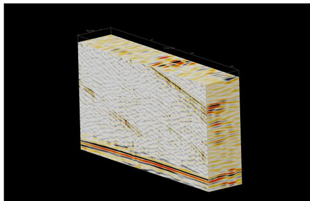
*Fig. 10. 3-D data volume showing two fractures of dip angle of 25 degree.*
