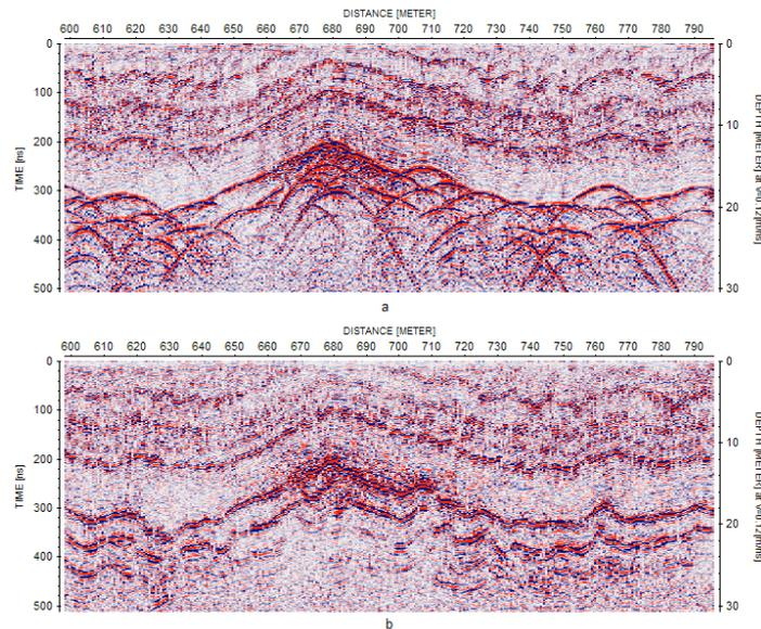
*Fig. 9. Georadar section before (a) and after 2-D Kirchhoff time migration (b).*
