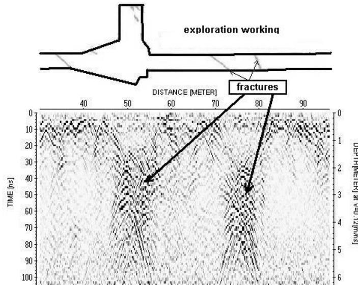
Fig. 19. 250 MHz GPR profile, acquired along the floor of exploration drift, shows the columns of diffraction hyperbolae that indicate the position of scattering points at sub vertical fracture surface.
