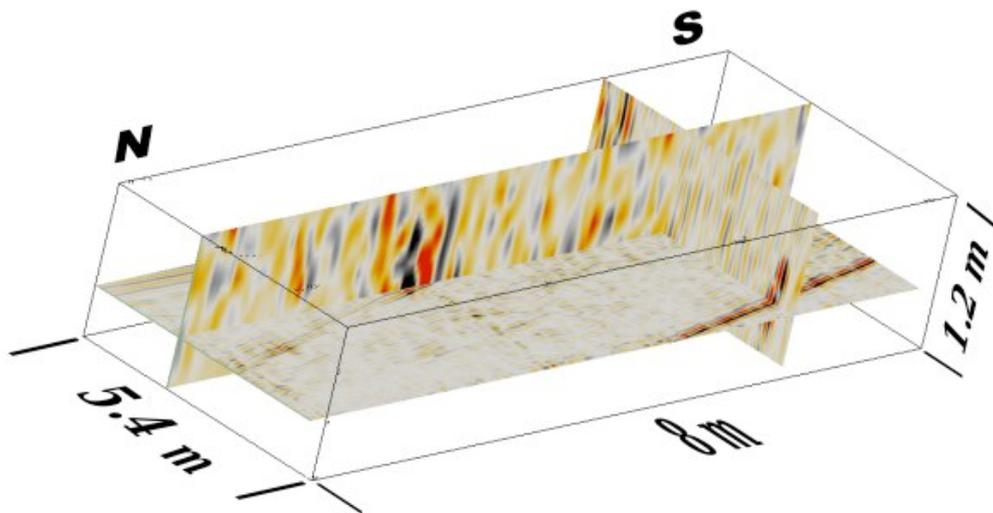
*Fig. 14. 3-D image of two fractures. Orientation of the data volume corresponds to side-look direction of sounding.*
