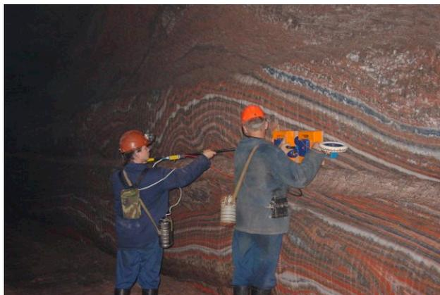
Fig. 7. Typical side-look profiling operations in Solikamsk mine 3 with OKO system.
