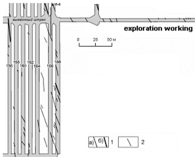
Fig. 18. Schematic map of fracturing distribution in the area of GPR survey: 1 – fractures detected by visual inspection of openings; 2 – fractures detected by georadar (Kudryashov et al, 2004).
