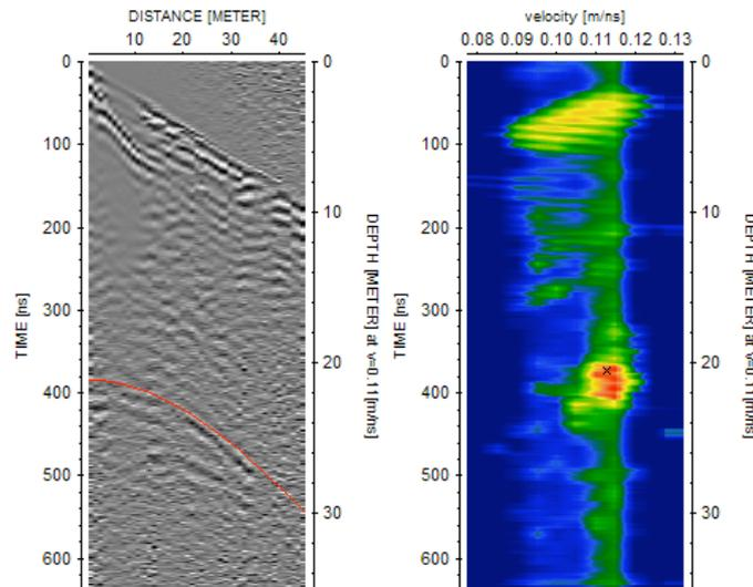
Fig. 11. Velocity semblance chart showing the velocity 0.11 m/ns for the underlying rock salt.
