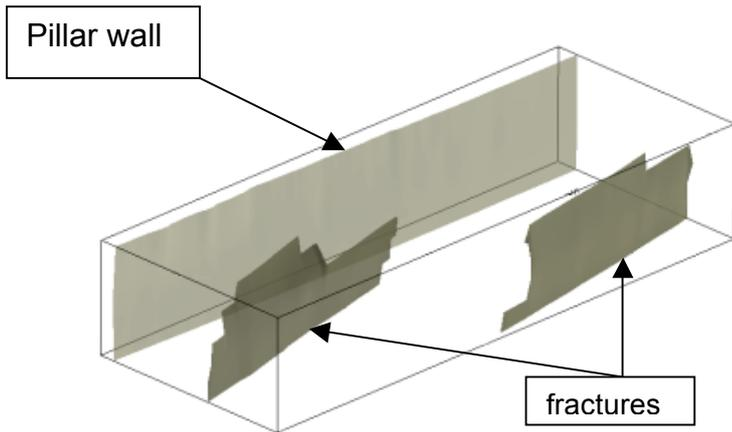
Fig. 15. Spatial model of two fractures into the pillar derived from the 3-D georadar data.
