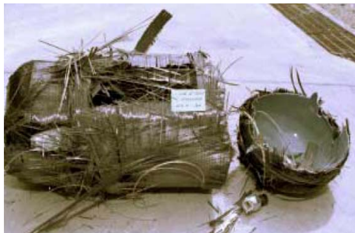
Figure 15. Composite over wrapped tank after hydrostatic burst test [26].
