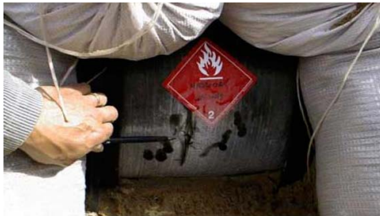
Figure 13. Cylinder subjected to gunfire test with no observable fragmentation [24].
