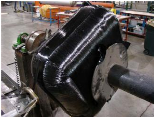
Figure 12. Pillow shaped pressure tank [22].
