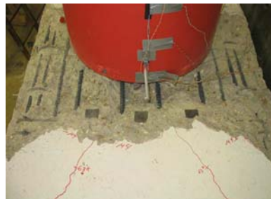
(c) Bent Cap Damage
