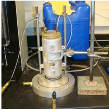
(a) Use a different split mold to hold the silt specimen and fix the specimen with a holder
