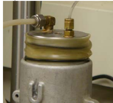
(f) Change a filter paper and set the GCTS cap with screw
