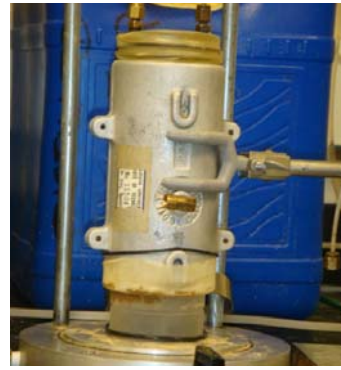
(b) Move away o-rings and stretch up the membrane
