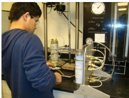
(g) Put vacuum at the top and bottom of the specimen to remove the air and move away the split mold
