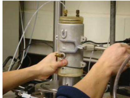
(d) Move the silt specimen to the GCTS platen and fix it with the holder
