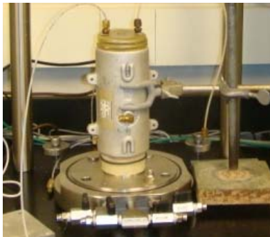
(e) Stretch down the membrane and o-rings to the GCTS base
