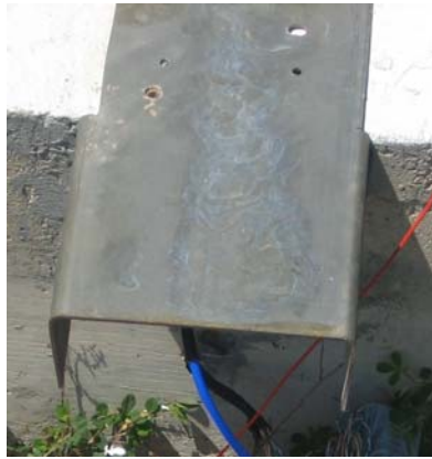
Figure 4.4. Steel Plate to Protect Sensor Connectors
