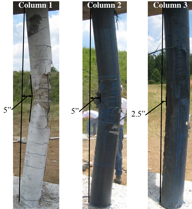
Figure 5.3. Comparison of Permanent Deflections
