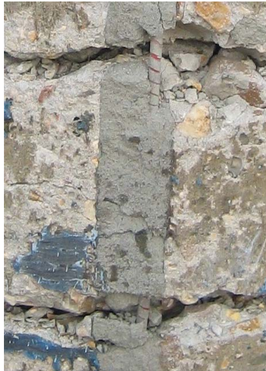
Figure 2.3. Separation of Steel Spirals in Two Cracks
