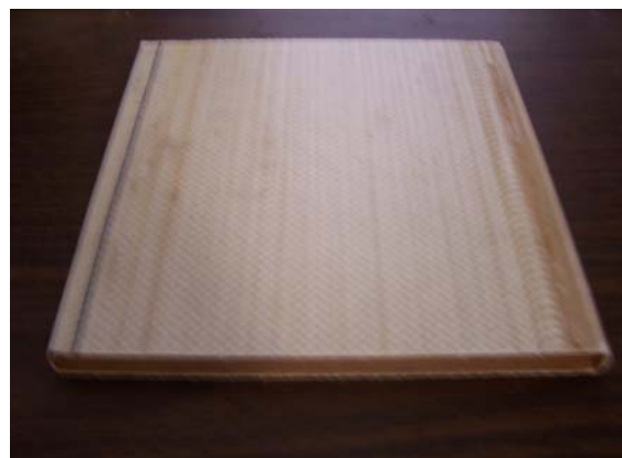
Figure 11. Core-filled Composite Manufactured at Missouri S&T
