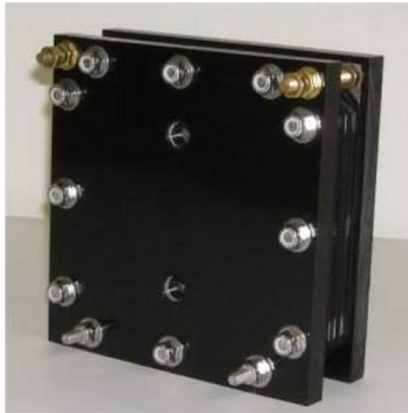
Fig 5: End Plates for fuel cells <sup>[6]</sup>
