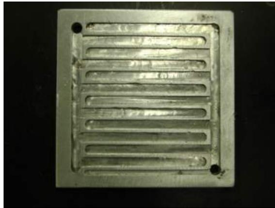
Fig 18: The machined bipolar plate with inter-digitated flow field design
