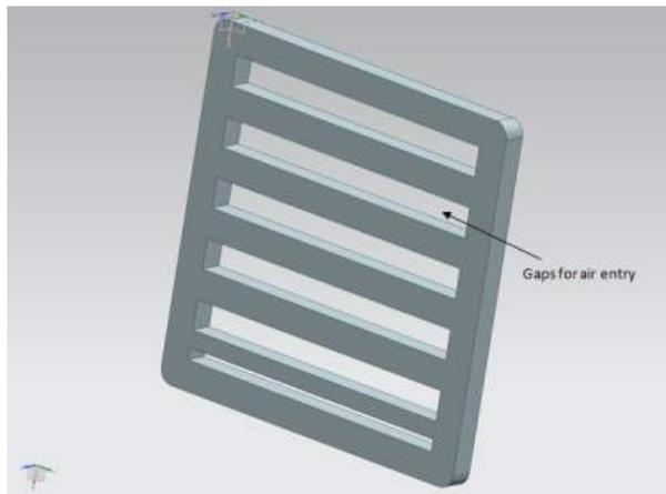
Fig 19: Open ended cathode plate
