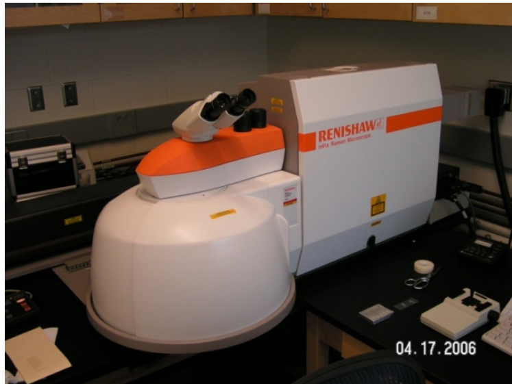
Figure 3-1. Multi-laser Renishaw Raman spectrometer.
