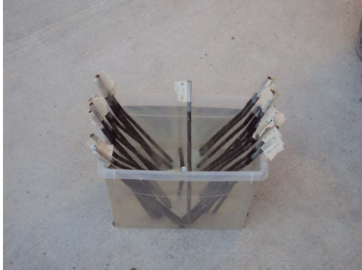
Figure C- 112 Steel Tendons Immersed in Muriatic Acid Solution
