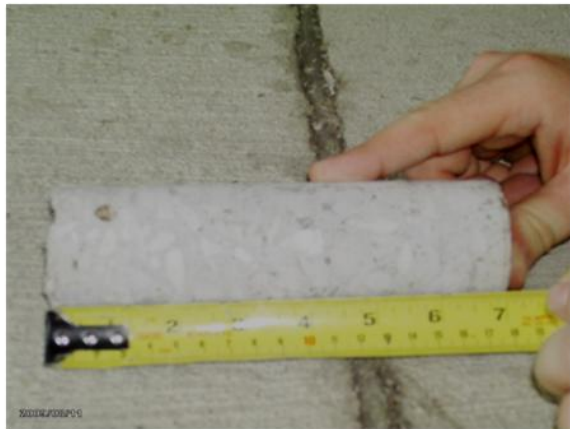
Core C-9: 7" long (broken)
