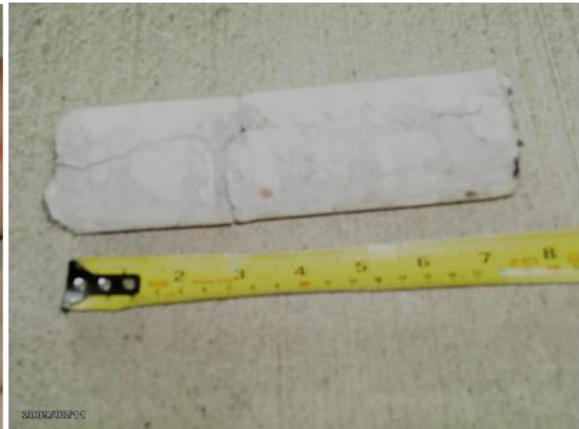
Core C-10: 7.125" long (broken)
