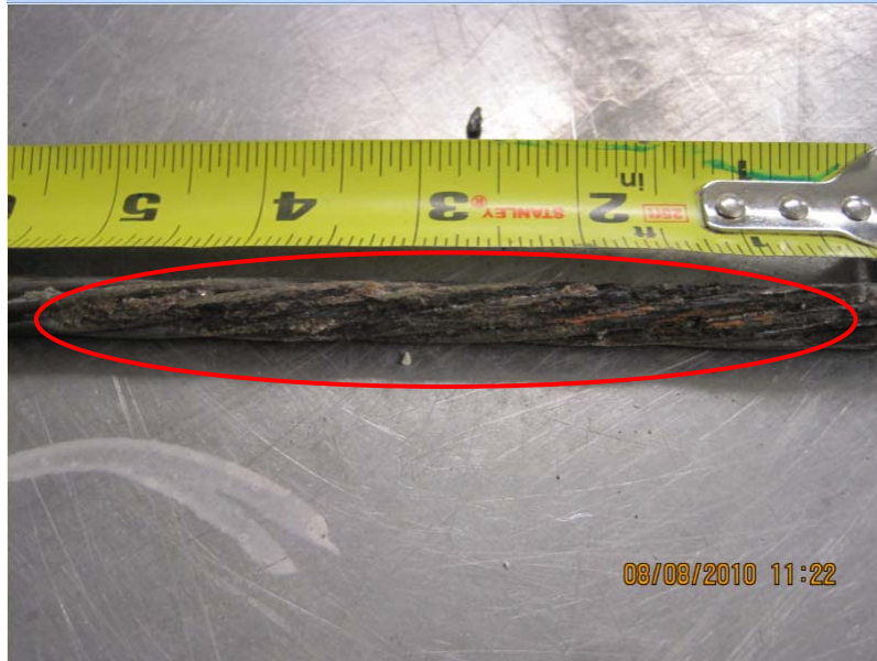
Figure 5-49 Example of Corrosion Area (SP1-FRC-13)
