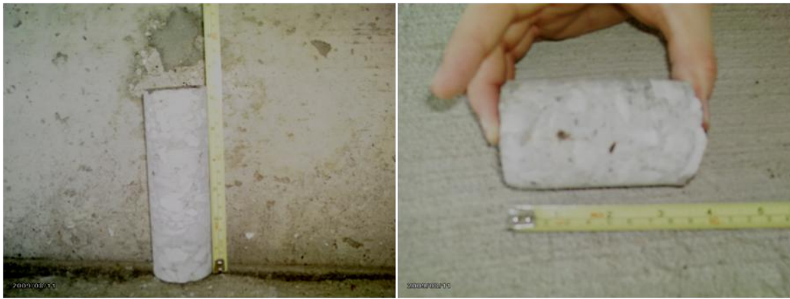
Core C-3: 6.125" long (smooth) Core C-4: 6.125" long (smooth)
