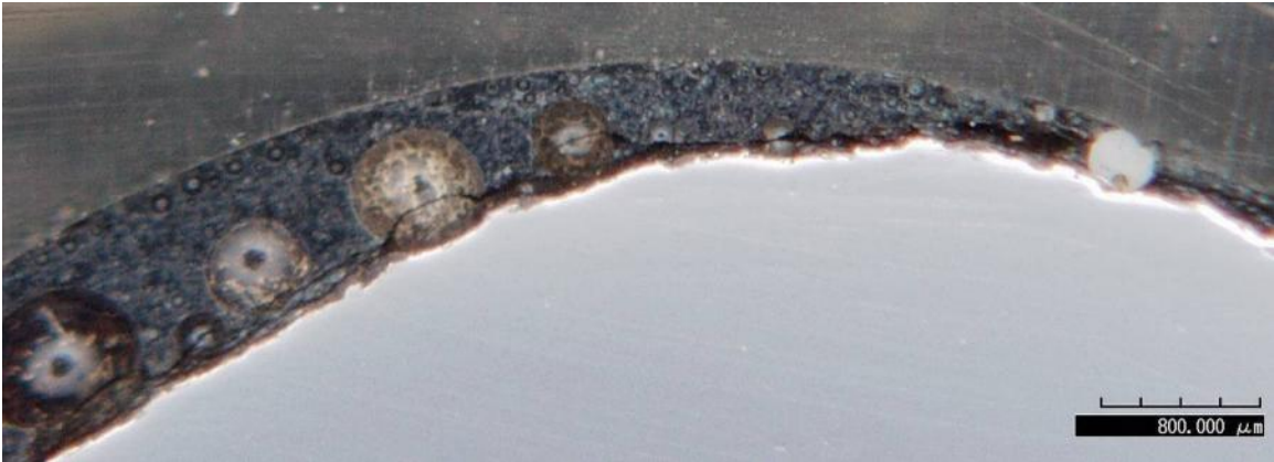
(b) Thickness variation of coating in a deformed bar
