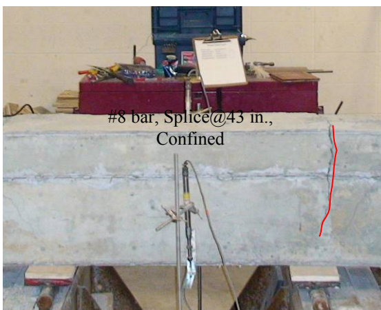
(k) Flexural failure of B-8-3
