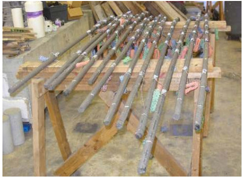
(a) Strain gauges on main reinforcement
