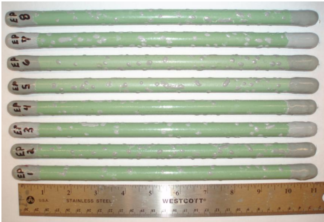
Figure A - 20: Front side of the smooth epoxy-coated salt spray specimens after testing.
