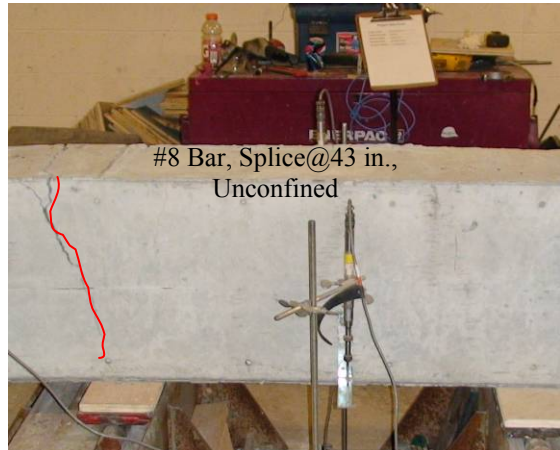
(l) Flexural failure of B-8-4
