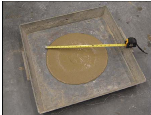
Figure 5-2: Measurement of CLSM flow
