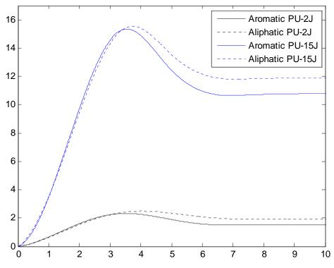
Figure 5. Energy vs time plot for glass reinforced PU composites
