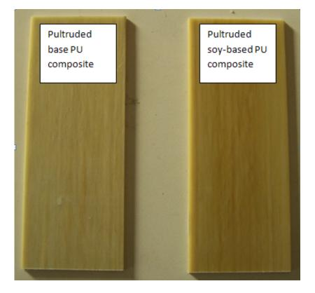
Figure 1. Pultruded parts manufactured at Missouri S&T
