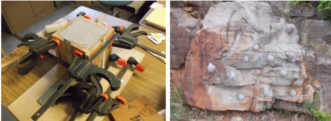
Figure 14: Clay pressed into a mold with a volume of 3706 ml (left) and the clay attached to the rock outcrop simulating 9 individual blocks.
