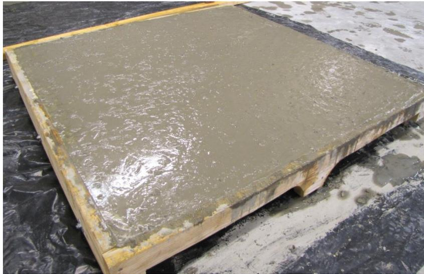
Figure 4.4. Completed LCFRC Impact Panel In Formwork
