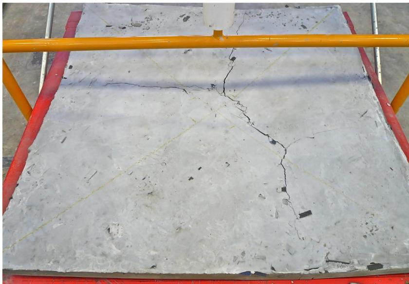
Figure 4.12: Typical Top of Fiber B1 Panel Failed Specimen
