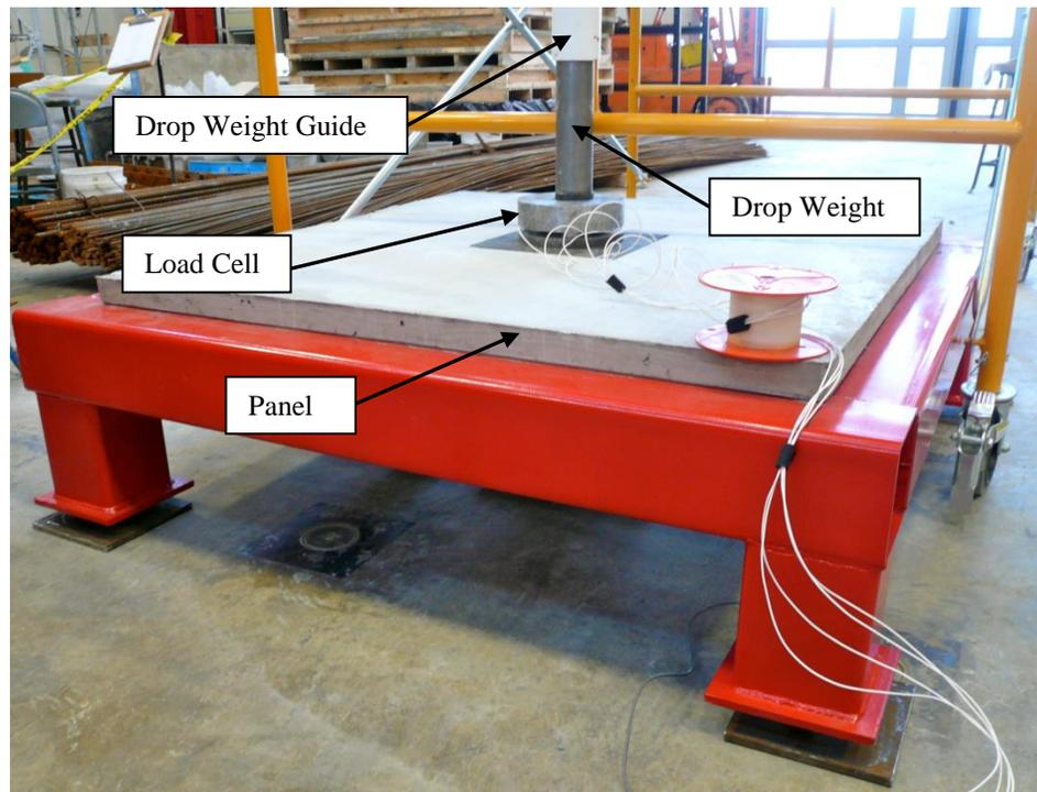
Figure 4.5: Drop-Weight Impact Test Setup
