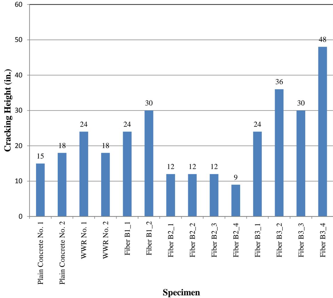
Figure 4.8: Summary of Cracking Heights for Drop-Weight Impact Testing
