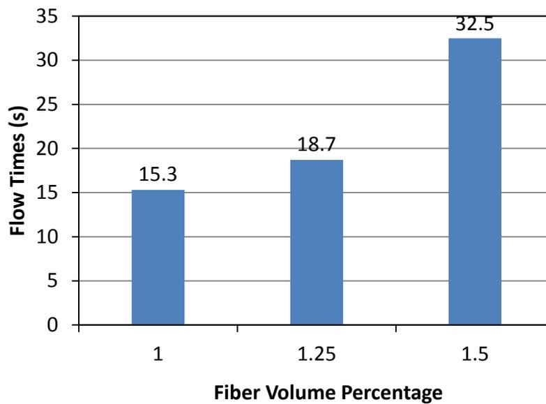
Figure 3.2. Flow Cone Test Results (ASTM C995)
