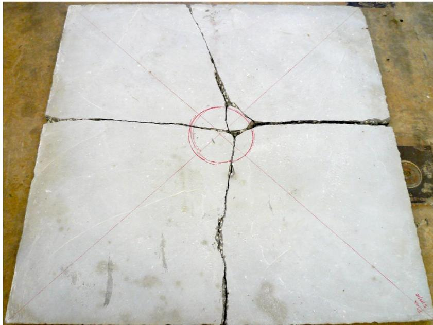
Figure 4.10: Typical Top of Plain Concrete Panel Failed Specimen
