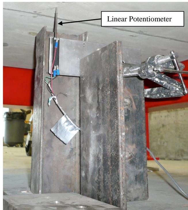
Figure 4.7: Linear Motion Potentiometer Setup
