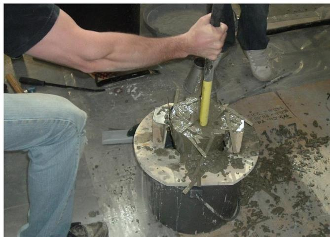
Figure 3.1. ASTM C995 Fiber- Concrete Flow Cone Test
