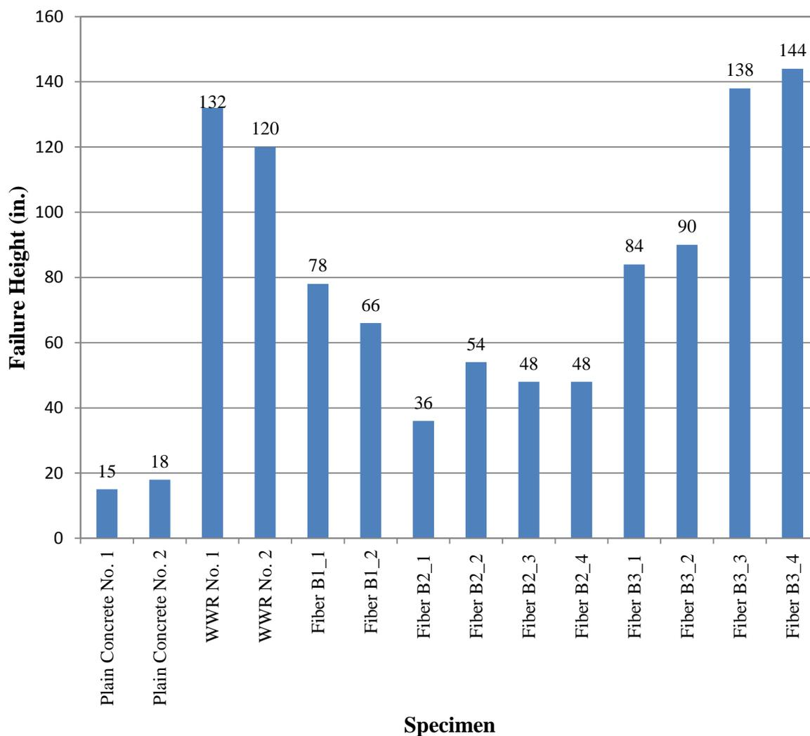
Figure 4.9: Summary of Failure Heights for Drop-Weight Impact Testing
