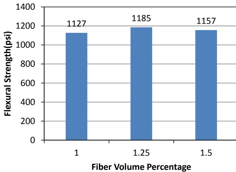
Figure 3.3. Flexural Strength Test Results (ASTM C78)
