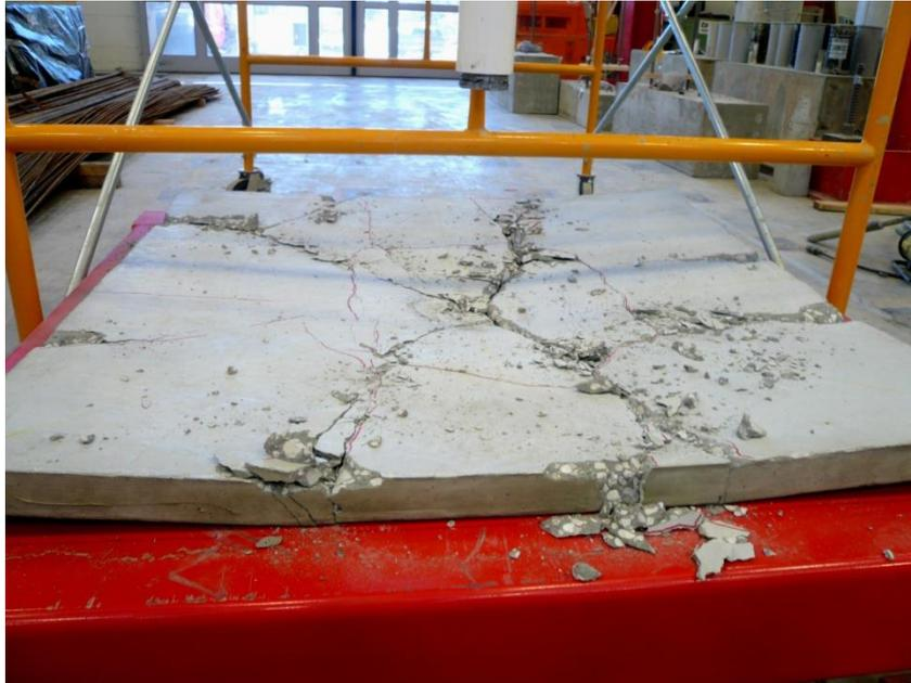
Figure 4.11: Typical Top of WWR Panel Failed Specimen
