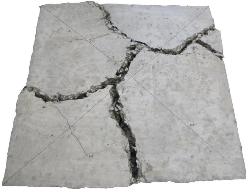
Figure 4.13: Typical Top of Fiber B3 Panel Failed Specimen
