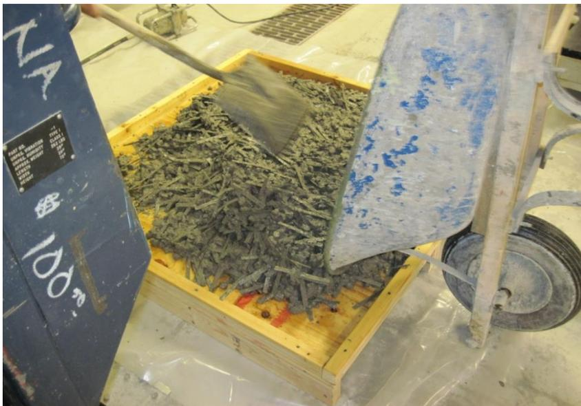
Figure 4.3. LCFRC Impact Panel Construction
