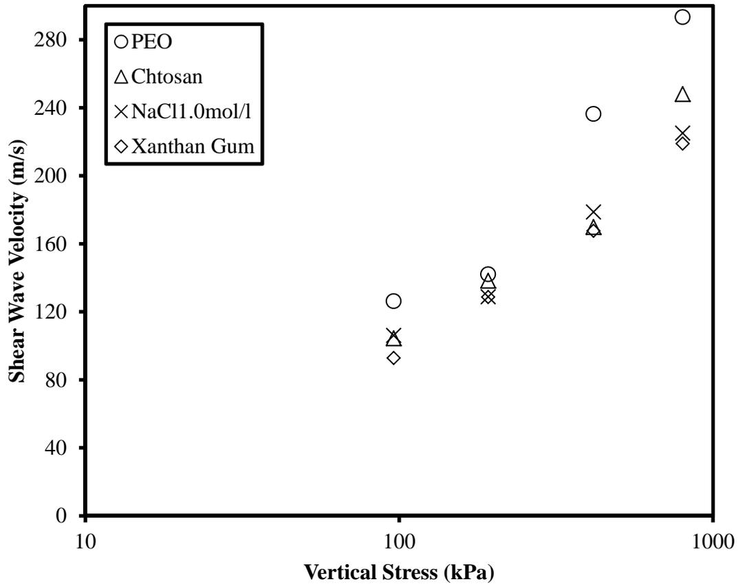
Figure 6 the  $V_s$  change in hh direction of kaolinite samples at different polymers and salt concentrations (PEO, Xanthan Gum, and Chitosan at 1.0g/l)
