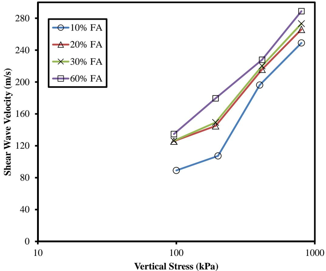
Figure 10 the  $V_s$  in hh direction of fly ash soil mixtures at different fly ash content during loading condition
