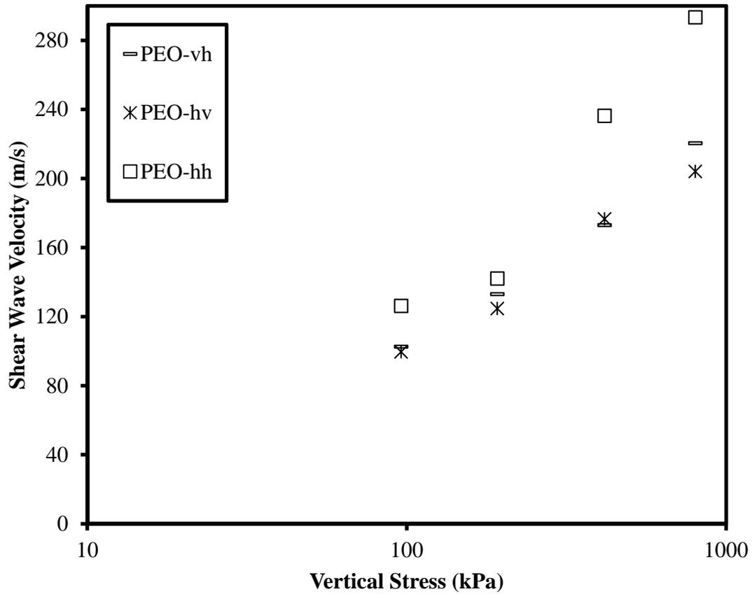
Figure 8 the shear wave velocity of PEO treated kaolinite sample in vh, hv, and hh directions during loading stage under virgin consolidation.
