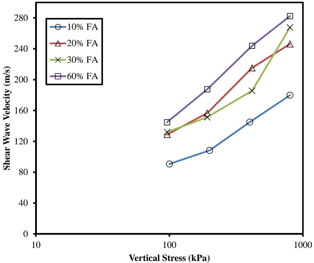
Figure 9 the  $V_s$  in vh direction of fly ash soil mixtures at different fly ash content during loading condition
