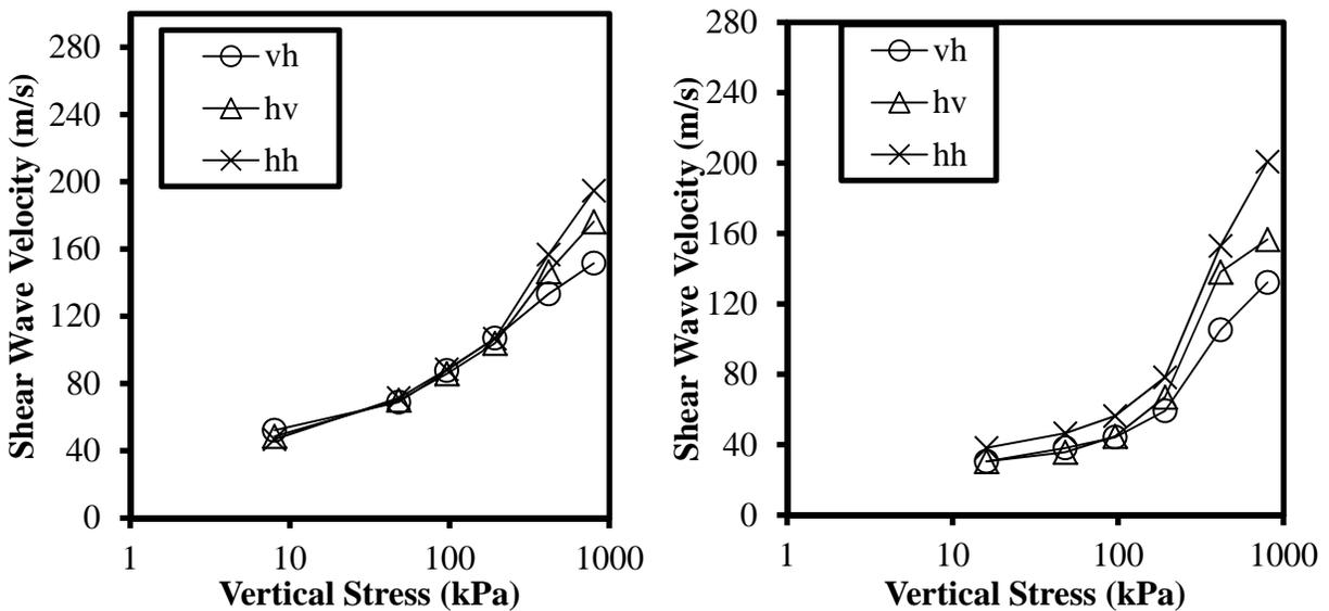
Figure 5 shear wave velocity in vh, hv, and hh directions of kaolinite samples at 1.0 mol/L and 0.01mol/L NaCl salt concentration during loading stage
