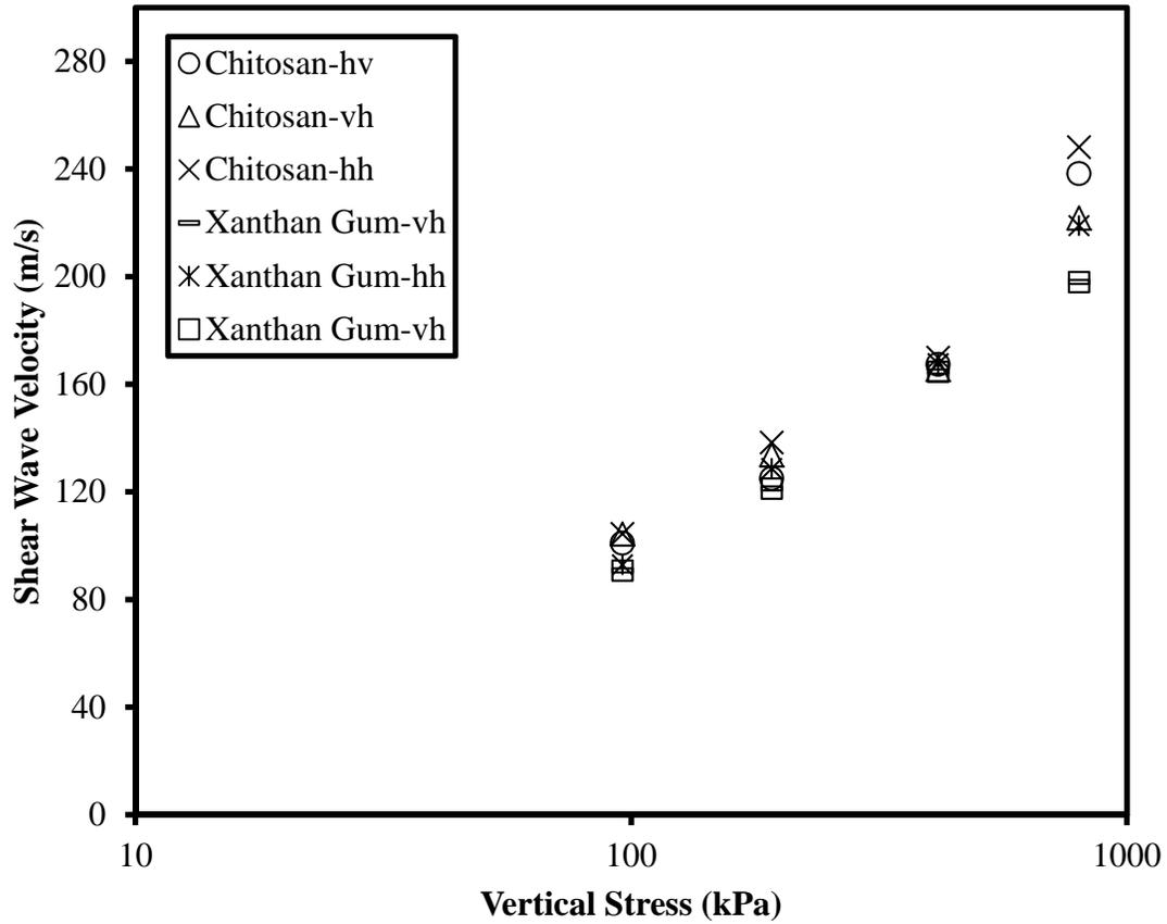
Figure 7 the shear wave velocity of Chitosan and Xanthan Gum treated kaolinite sample in  $vh$ ,  $hv$ , and  $hh$  directions during loading stage under virgin consolidation.
