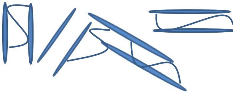
Limited polymer bridging, and aggregation induced by Xanthan Gum, dispersed and deflocculated structure.
