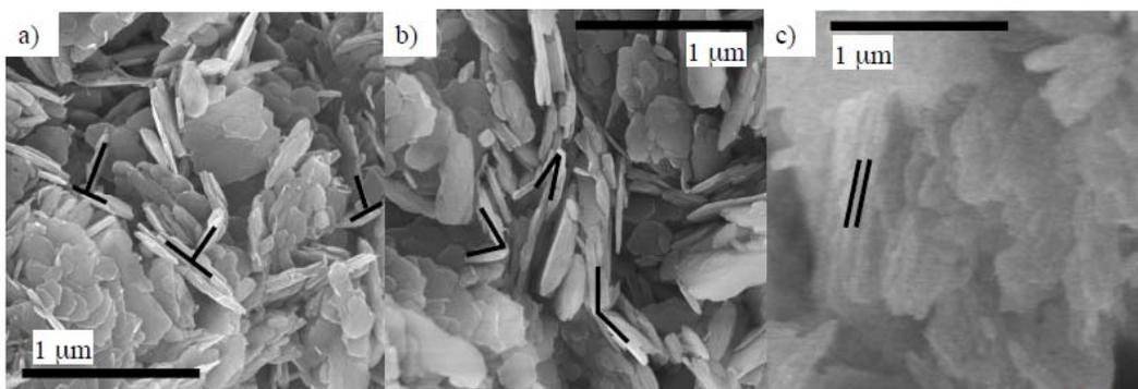
Figure 2. Scanning electron microscopy (SEM) images of Georgia 1 RP-2 kaolinite particles at a) 0.003 mol/l, b) 0.02 mol/l, and c) 1 mol/l of NaCl solutions. The corresponding fabric
