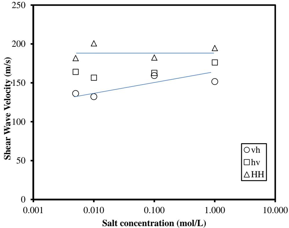
Figure 3 The shear wave velocity change in vh, hv, and hh directions of kaolinite samples at different NaCl concentrations under a nominal consolidation stress of 800kPa
