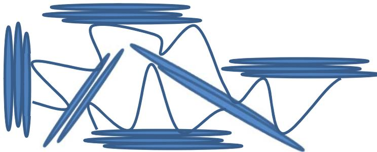
Charge neutralization induced aggregation and polymer bridging induced flocculation by Chitosan
