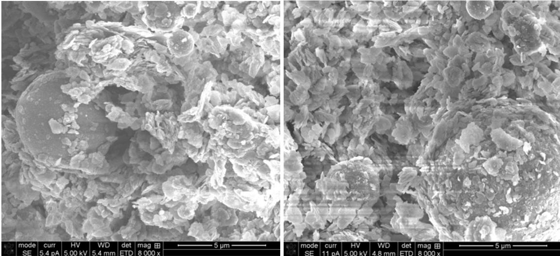
Figure 14 SEM images of fly ash soil mixture with a mixing ratio of 30%FA+70%KA
