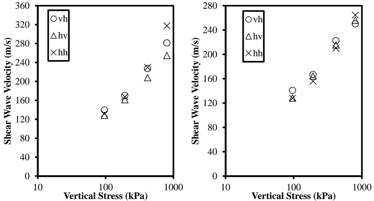
Figure 12 the  $V_s$  of PEO and Chitosan where is xanthan? modified fly ash soil mixtures in vh, hv, and hh directions
