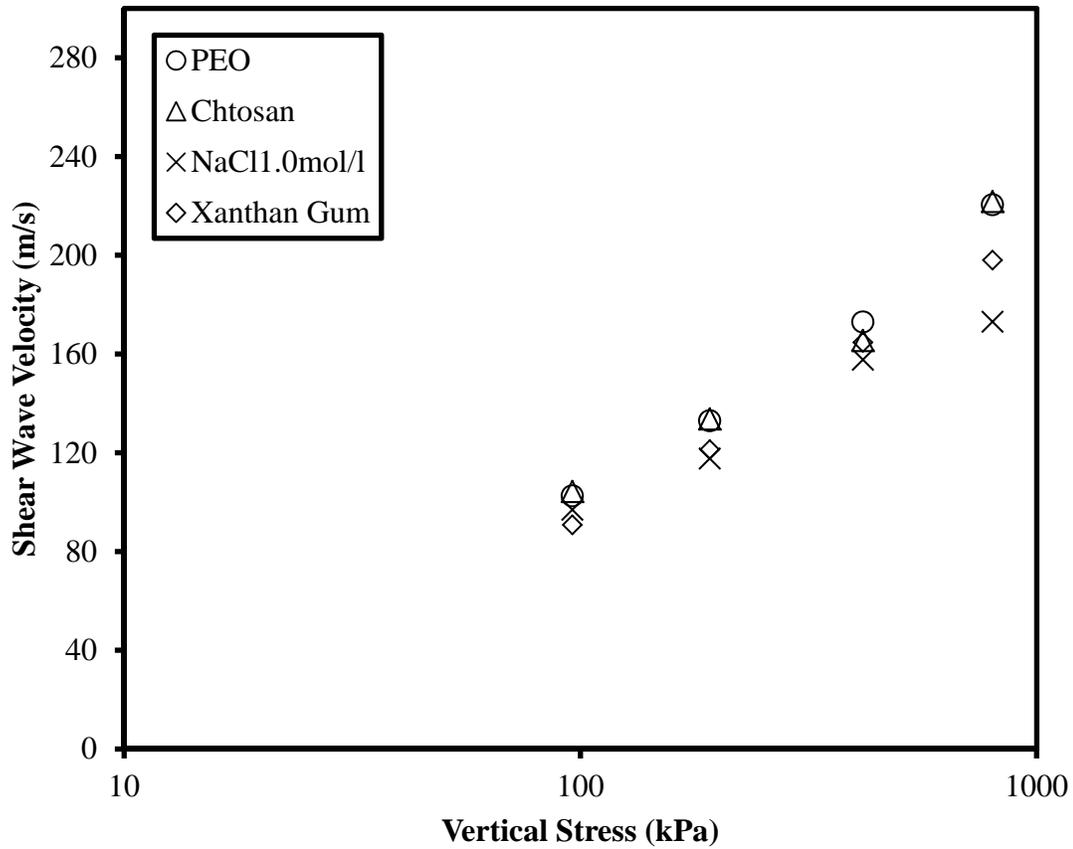
Figure 15 the  $V_s$  change in hh direction of kaolinite samples at different polymers and salt concentrations (PEO, Xanthan Gum, and Chitosan at 1.0g/l)
