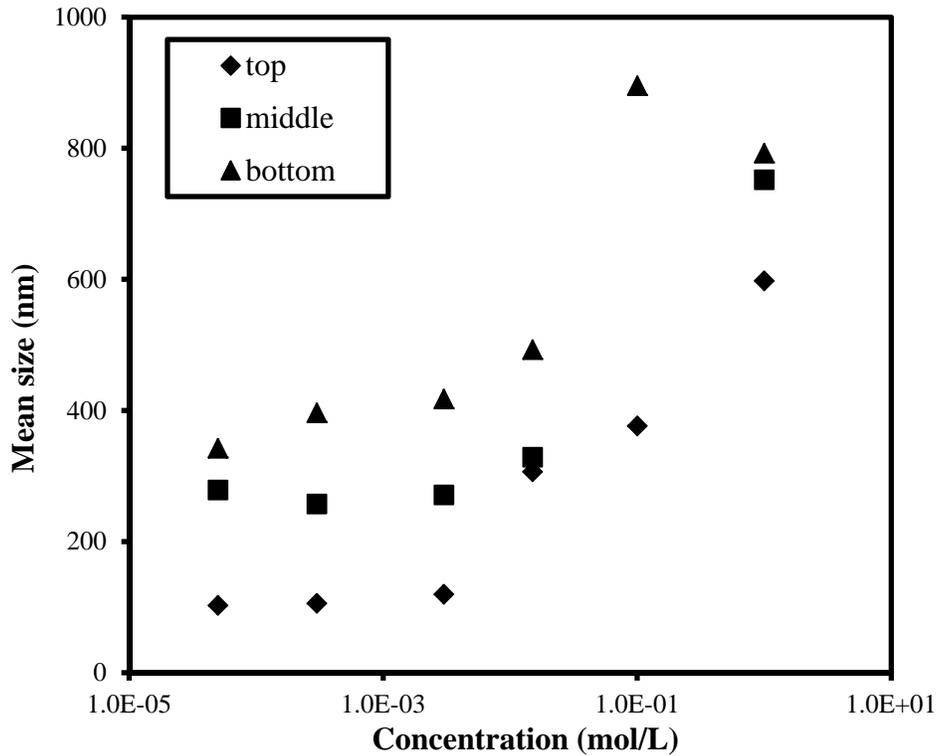
Figure 16 Grain Size Distribution of Kaolinite Flocs at different Salt Concentrations
