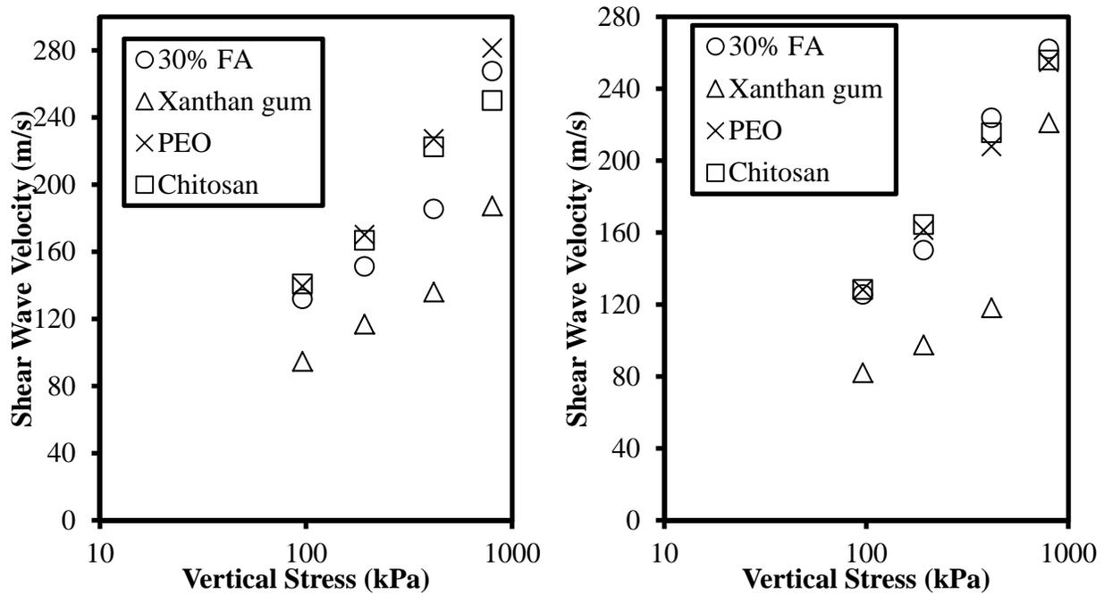
Figure 11 the  $V_s$  of organically modified fly ash soil mixtures in vh and hv directions
