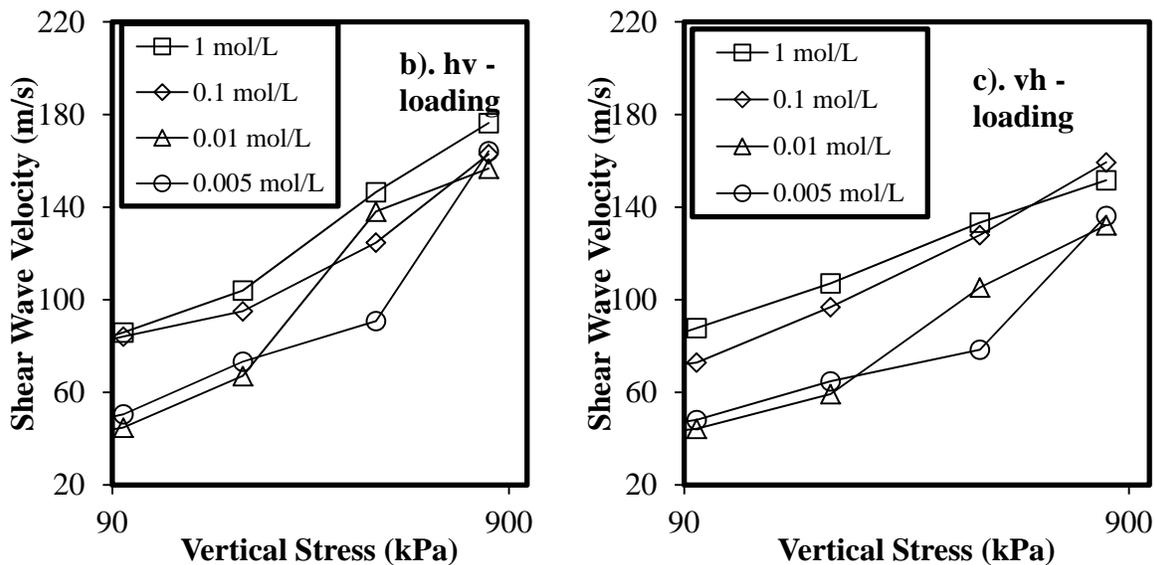
Figure 13  $V_s$  of kaolinite sample consolidated at different salt concentrations in vh, and hv directions
