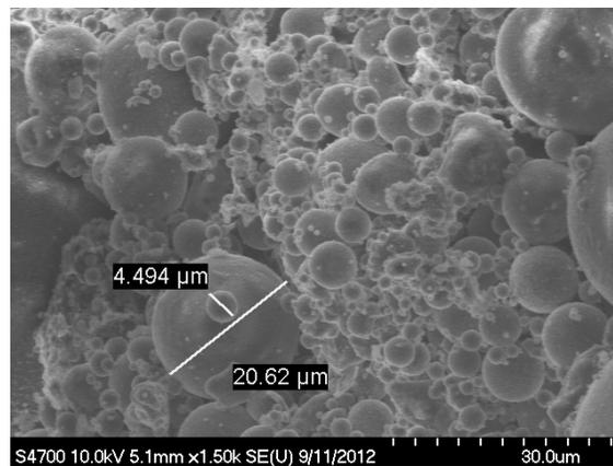
Figure 1 Fly Ash Particle Images under SEM (Lafarge, Wisconsin, Class F)
