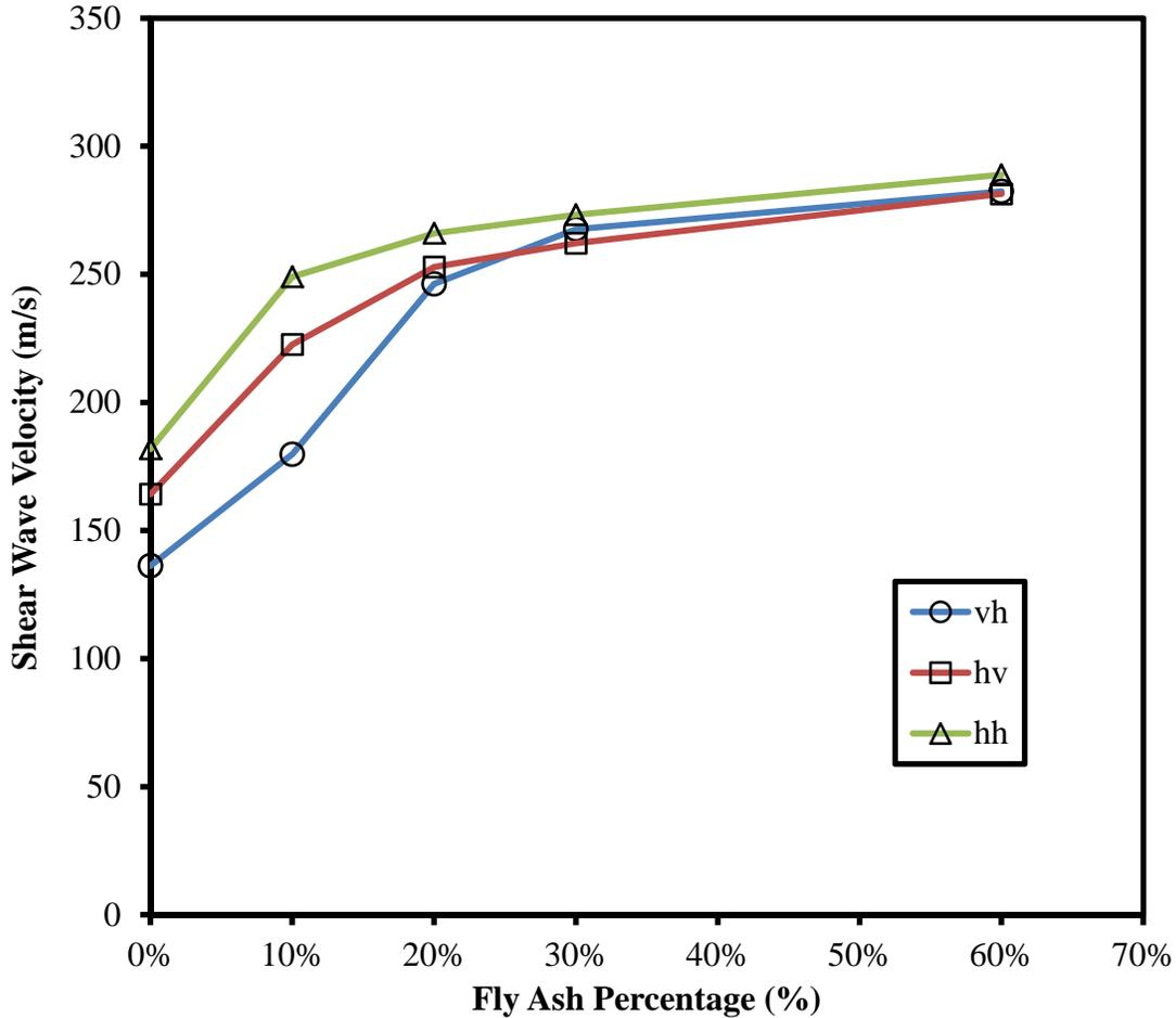
Figure 4 the shear wave velocity changes in vh, hv, and hh directions of fly ash kaolinite mixtures at different mixing ratios under a nominal consolidation stress of 800kPa
