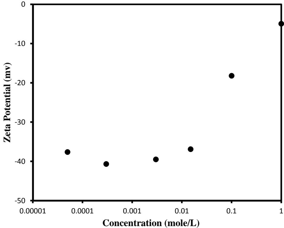
Figure 15 the zeta potential of Kaolinite at different Salt Concentrations
