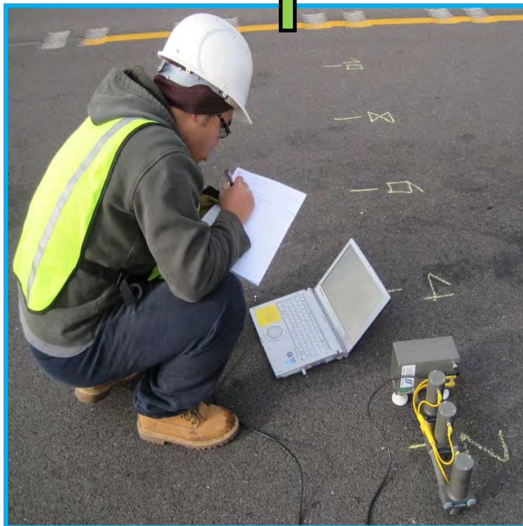
Figure 20. Portable seismic pavement analyzer data acquisition (PSPA).
