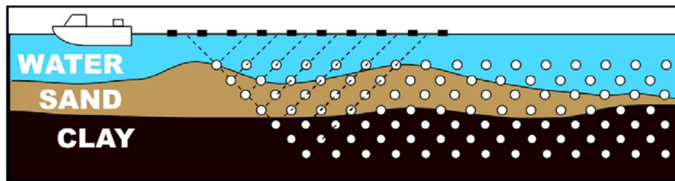
Figure 14: Sample setup of marine survey an array of electrodes towed behind a boat (Wei, 2011).
