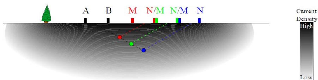
Figure 13: Multi-electrode dipole-dipole resistivity array (Frontier Geosciences, 2001).
