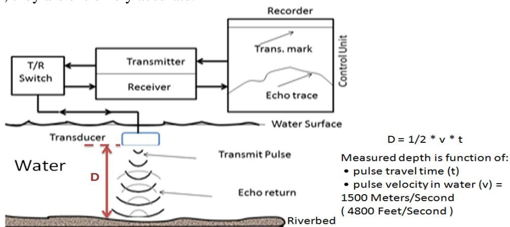
Figure 10: shows basic Echo Sounder Operation (Modified after Mueller & Landers, 1999).
