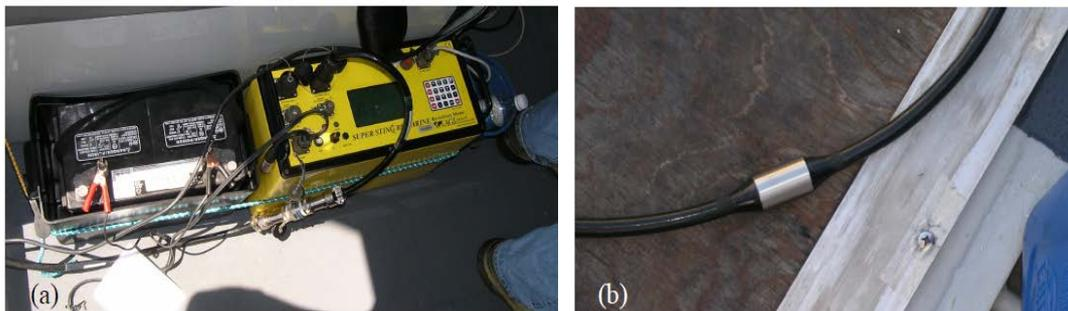
Figure 23: Equipment Photos (a) AGI Supersting Marine (b) stainless steel electrode on towed cable. (Enviroprobe Service, Inc.).
