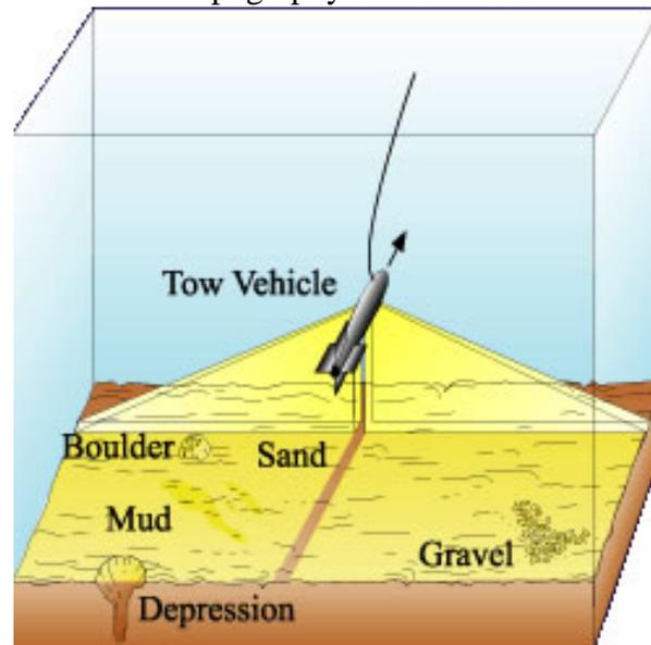
Figure 11: shows side scan sonar (Kvitek et al., 1999).
