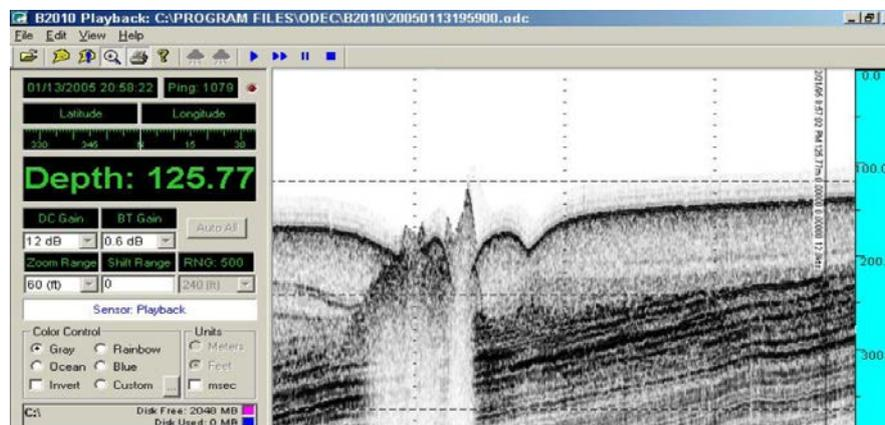
Figure 19: The sub bottom profiler and bathymetric acquisition software.
