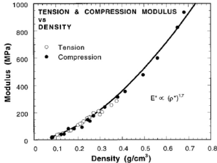
Fig. 6. Variations of the modulus of elasticity of typical foam with density. In the figure, the modulus of the closed cell foam varies as the 1.7 power of mass density. From S.H. Goods, C.L. Neuschwanger, L.L. Whinnery and W.D. Nix, “Mechanical Properties of a Particle-Strengthened Polyurethane Foam,” *Journal of Applied Polymer Science*, Vol. 74, pp. 2724-2736, 1999. Similar results have been published for open-cell foams, though the power was different.
