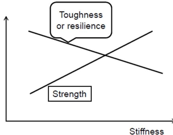
Fig. 2. Dual effect of higher stiffness: the strength of stiffer materials is usually higher, but their toughness and resilience are lower.
