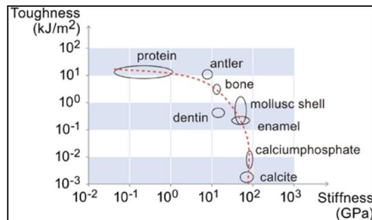
Fig. 1. Toughness of engineering (top figure) and biological (bottom figure) materials increases as their stiffness decreases. Accordingly, it is concluded that energy absorption increases in compliant materials.
