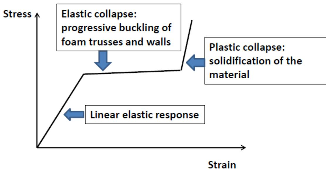
Fig. 5. Stress-strain relationships of typical foam. Absorbed energy is the area below the stress on the stress-strain diagram.
