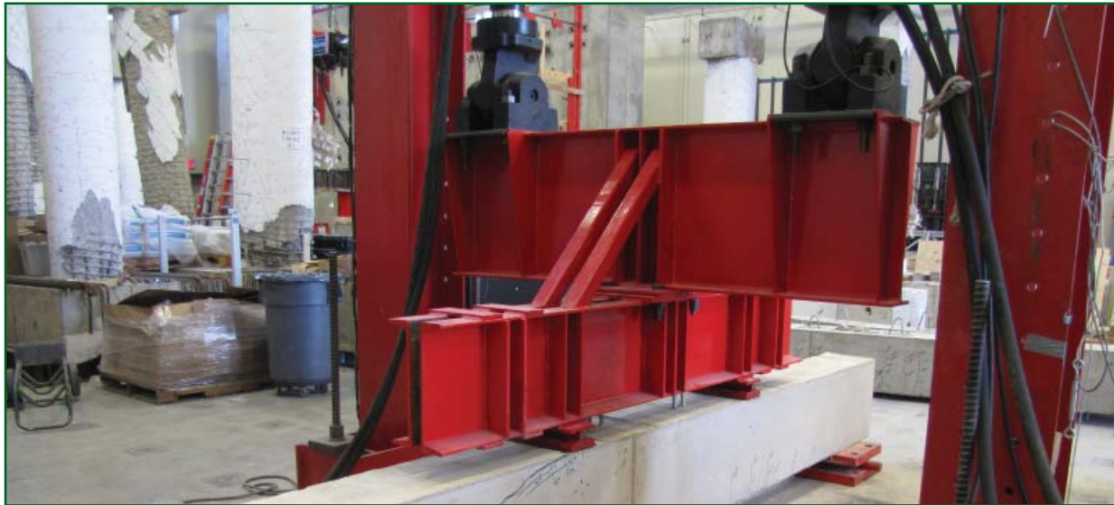
Figure 2. Full-scale beam shear test
