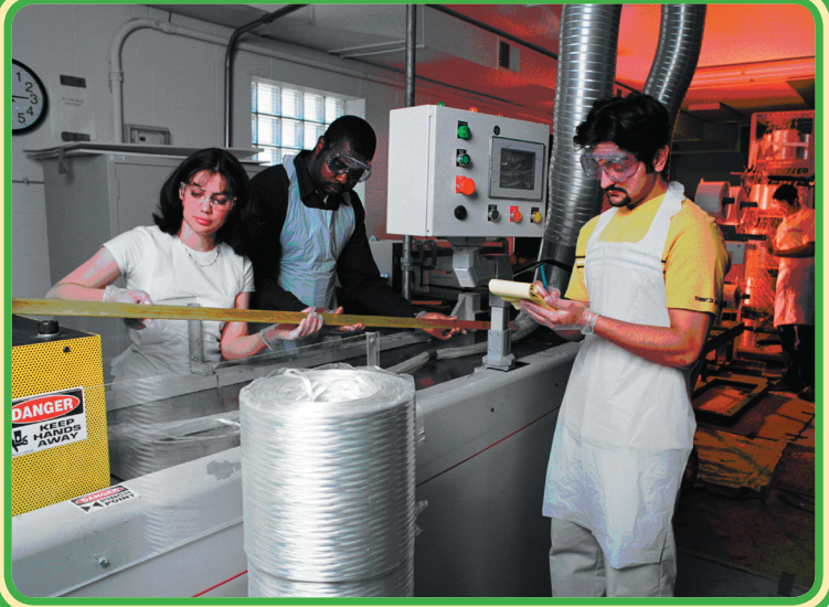
Students performing the pultrusion process at the Composite Manufacturing Laboratory at Missouri S&T.
