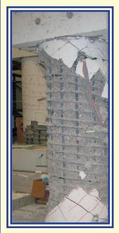
**NUTC-sponsored** project intends investigate the behavior of RC bridge columns when subjected to different kinds of load stresses, including combined axial, bending, shear and torsion both through experimental and analytical studies. Through this investigation, a direct interaction of bending, shear and torsion under constant axial load will be established and used to develop new design tools for engineers.
