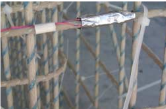
Figure 4. Strain gage on GFRP bar
