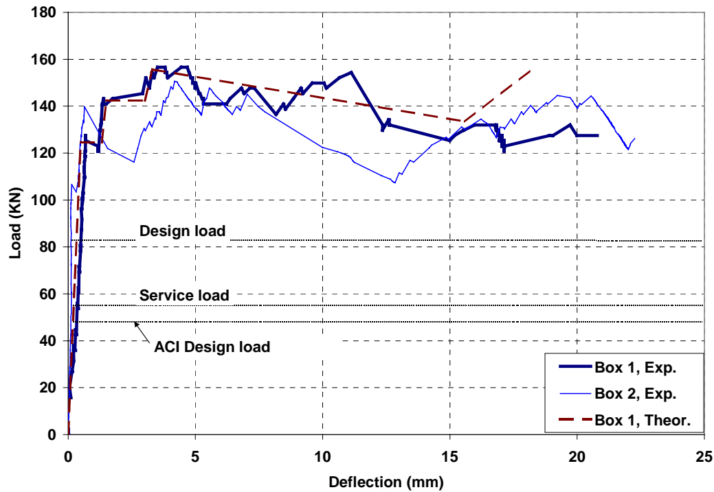
Figure 9. Comparison of experimental and theoretical load-deflection behavior
