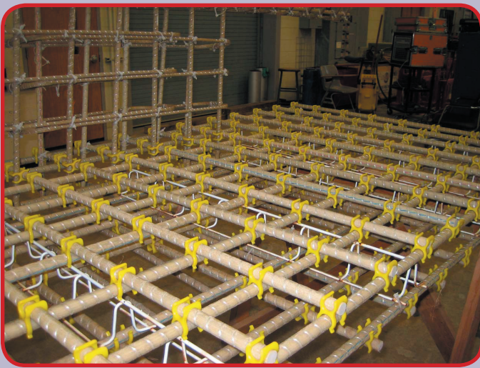
A steel free mock-up at the SERL High Bay Structures Lab.
